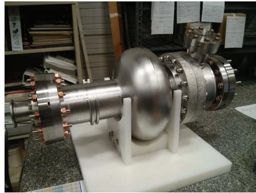
Figure 4: The quarter-wave coaxial coupler with a single cell cavity.
