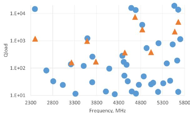
Figure 8: Comparison of CST  $Q_{load}$  and measured  $Q_{load}$  for the cavity with grooved beam pipe (200 mm). Circles – CST  $Q_{load}$ , triangles – measured  $Q_{load}$ .
