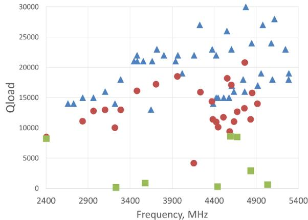
Figure 7:  $Q_{load}$  of the cavity with a grooved pipe length of the drift at the drift tube 400 mm. Triangles –  $Q_0$  calculation, circles -  $Q_0$  measurements, square -  $Q_{load}$  measurements.
