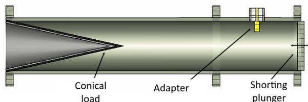
Figure 5: The scheme of the reflection coefficient measurements of the load.
