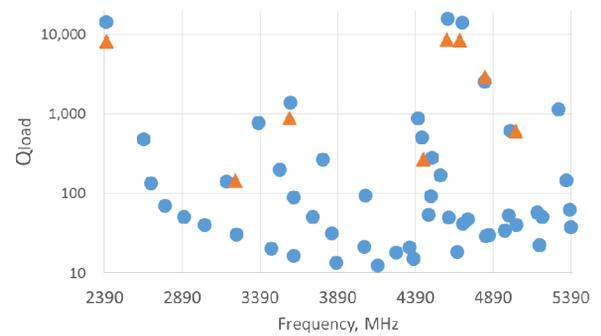
Figure 9: Comparison of CST  $Q_{load}$  and measured  $Q_{load}$  for the cavity with grooved beam pipe (400 mm). Circles – CST  $Q_{load}$ , triangles – measured  $Q_{load}$ .
