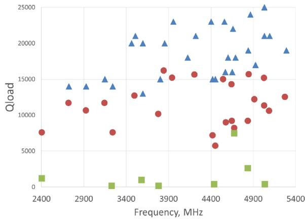
Figure 6:  $Q_{load}$  of the cavity with a grooved pipe length of the drift at the drift tube 200 mm. Triangles –  $Q_0$  calculation, circles -  $Q_0$  measurements, square -  $Q_{load}$  measurements.
