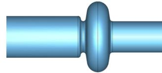
Figure 1: Cavity with grooved beam pipes.
