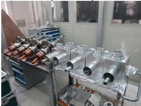
Figure 3: The fabricated coupler components.
