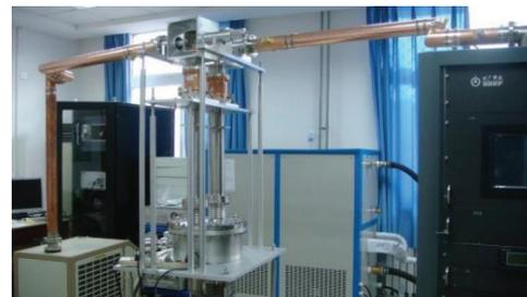
Figure 6: The high power test system for couplers of 325 MHz Spoke SCC.
