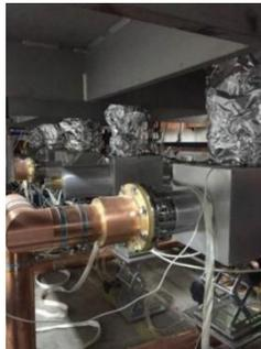
Figure 10: The in-situ input couplers of 162.5 MHz HWR-010 SCC for Injector-II.
