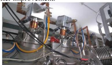
Figure 9: The in-situ input couplers of 325 MHz Spoke-012 SCC for Injector-I.
