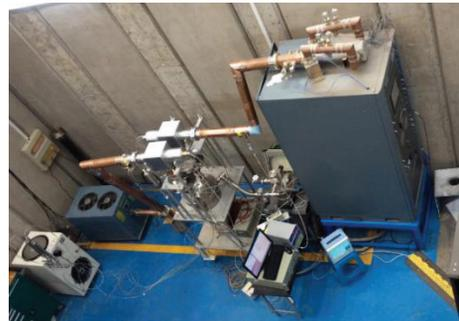
Figure 5: The high power test system for couplers of 162.5MHz HWR SCC.
