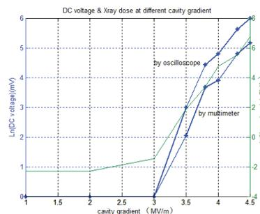
Figure 8: The DC voltage and X-ray dose at different cavity gradients.
