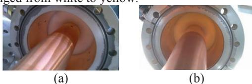
Figure 7: The vacuum side of the window: (a) before assembled in the cavity; (b) after disassembled from the cavity.
