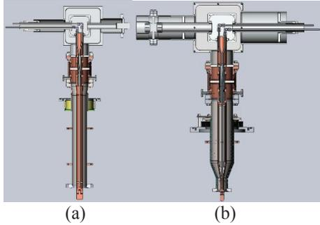
Figure 2: The general layout of high power input couplers for C-ADS: (a) Spoke-012 SCC input coupler; (b) HWR-010 SCC input coupler
