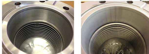
Figure 6: Nb-coated (left) and Nb-on-Cu (right) welded bellows.
