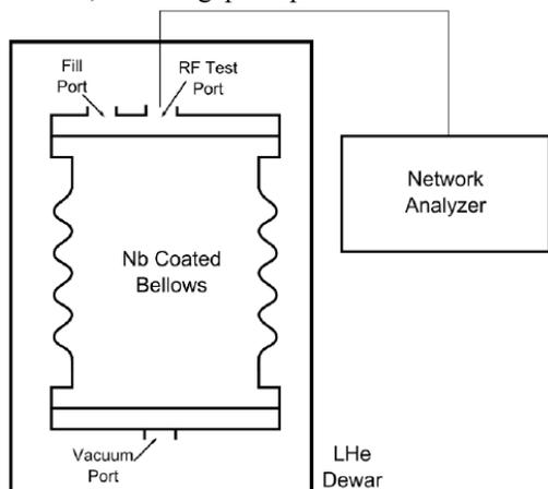
Figure 4: Schematic of coated bellows cavity test.
