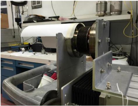
Figure 7: Bellows cycling device.
