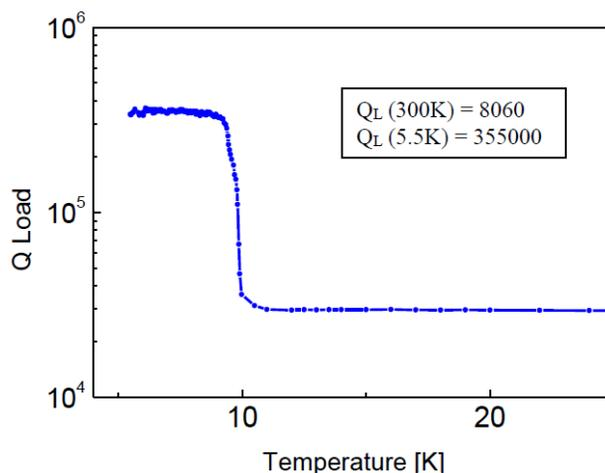
Figure 5:  $Q_L$  of bellows cavity vs. temperature.
