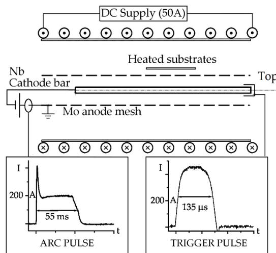
Figure 1: CED process schematic drawing.
