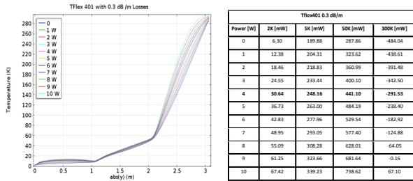
Figure 6: Cable choice for LCLS-II CM. (a) Temperature distribution. (b) Thermal intercepted power by cooling.
