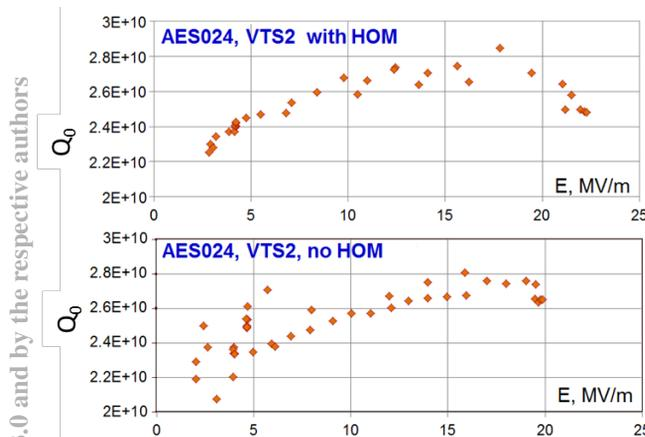
Figure 7: Experimental testing of TB9AES024:  $Q_0$  vs E for the cavity with and w/o HOMs.
