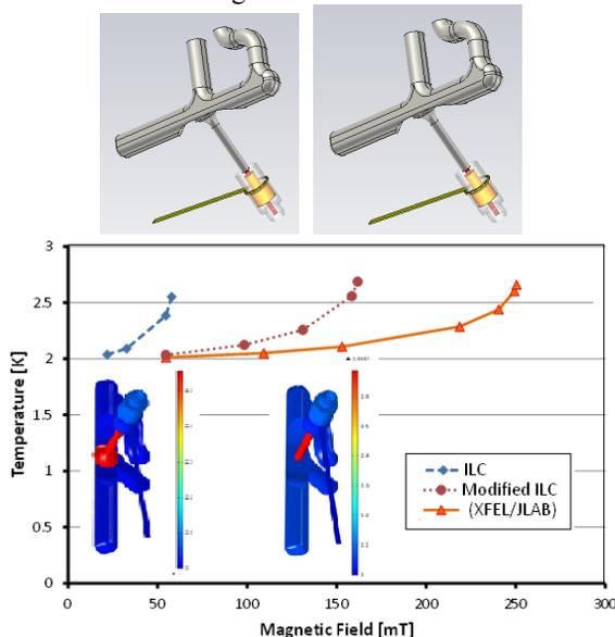
Figure 4: Thermal analysis of both (a) the conventional ILC antenna (b) and the modified one. (c) Temperature versus magnetic field for the ILC design, modified ILC design, and XFEL/JLAB design with ILC antenna tip.
