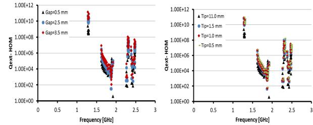
Figure 3: Effect of modifying the HOM antenna on external quality factor. (a) Effect of gap size. (b) Effect of tip size.
