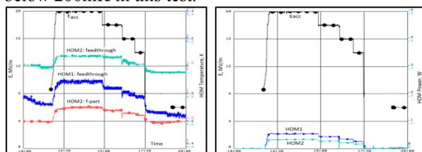
Figure 10: (left) - Temperature of the HOM coupler and feedthrough and cavity gradient. (right) – HOM power.
