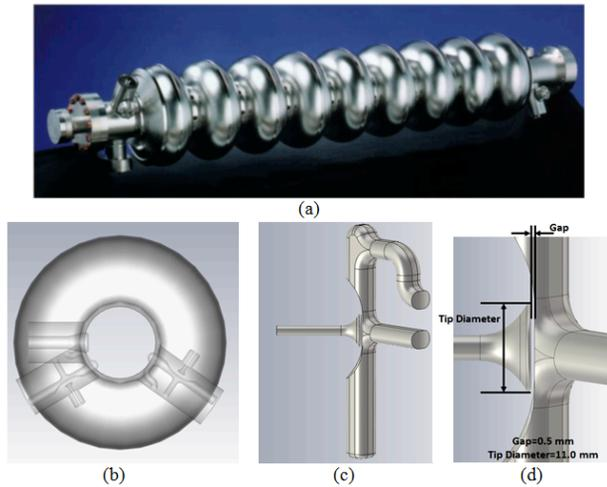
Figure 1: The geometry of the HOM coupler and antenna (a) ILC cavity. (b) Transparent front view of the cavity showing HOM couplers. (c,d) HOM antenna and f-part.
