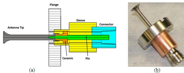
Figure 2: HOM coupler feedthrough. (a) Sketch showing the cross-section and highlighting the different feedthrough parts. (b) DESY feedthrough.
