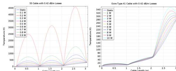
Figure 5: Performance of SS vs copper cables. (a) SS cable temperature distribution under various power flow conditions (up to 0.9W) (b) copper cable temperature distribution under various power flow (up to 10 W).
