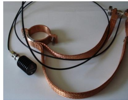
Figure 8: Copper braids for thermal connection of the HOM feedthrough to the 2K two-phase pipe in a cryo-module.
