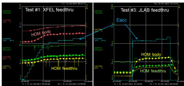
Figure 9: Test results for XFEL feedthroughs  $\sim 1^\circ\text{K}$  rise on HOM body and  $\sim 0.5^\circ\text{K}$  on feedthrough (left). Test results for JLAB-type feedthroughs:  $\sim 2.7^\circ\text{K}$  rise on HOM body,  $\sim 0.85^\circ\text{K}$  on feedthrough (right).
