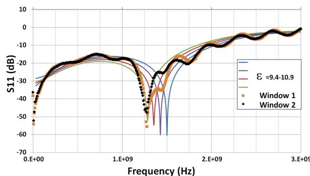
Figure 3: Measured (black and orange dots) and calculated reflection coefficients for two RF windows with the ‘hourglass-shaped’ central conductor
