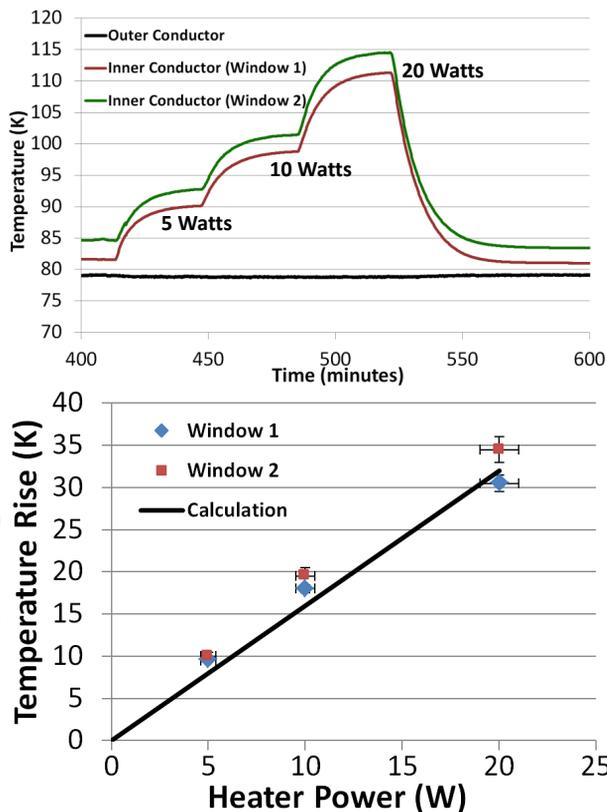
Figure 5: Top – temperature rise due to conduction in alumina and copper, bottom – analytically calculated versus measured temperature increase.
