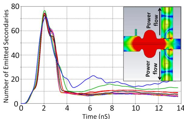
Figure 2: Main figure – CST multipacting simulations for several coupler RF power levels up to 50 kW CW (travelling wave). Inset – travelling wave due to coupling to the cavity electric field (red).
