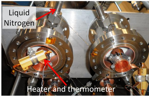
Figure 4: Calorimetry hardware for heat transfer measurements in RF windows at 80 K and 300 K
