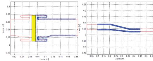
Figure 7: The window (left) and coaxial line (right) geometries for multipacting simulation. The blue dots are initial electrons.
