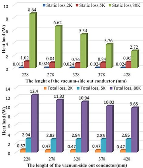
Figure 4: The static loss and total loss of 2 K flange, 5 K anchor and 80K anchor as the out conductor varies in different length with 150 kW power transmitted through.
