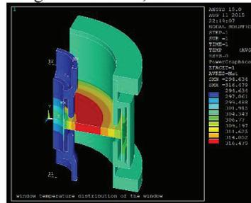
Figure 5: Temperature contour of the RF window at 300 kW, CW. Both the inner conductor cooling water temperature is and the window cooling air temperature is 20 °C.
