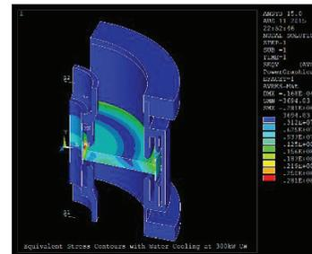
Figure 6: Stress contour of the window at 300 kW, CW.
