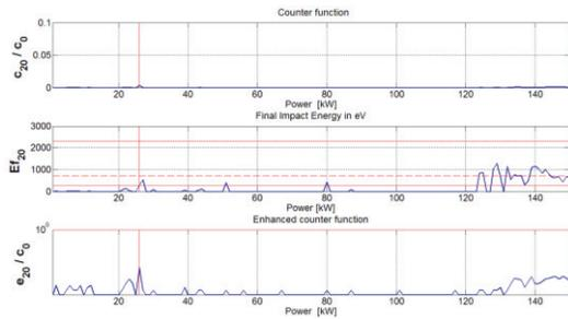
Figure 8: From the top to the bottom, the electron counter, the average impact energy of the last impact in eV and the enhanced electron counter in the coax line with a taper for a standing wave.
