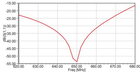
Figure 3: Calculated S11 parameter of the coupler
