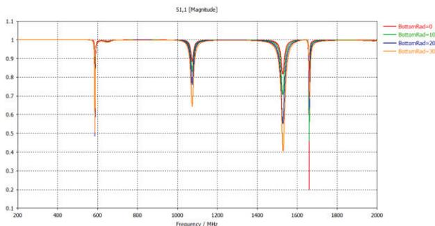
Figure 13: Variation in the narrow radius of the conical absorber.
