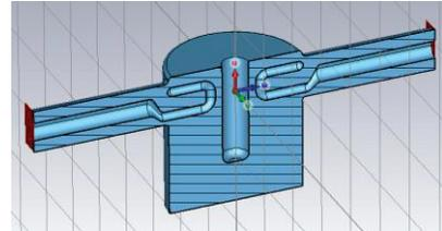
Figure 8: Final design for the RFD FPC test box.
