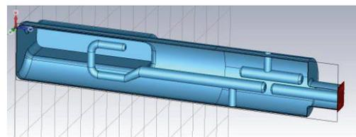
Figure 17: The horizontal HOM coupler for the RFD crab cavity.
