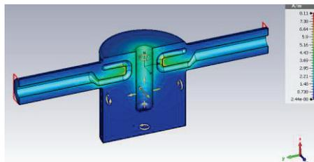
Figure 10: Magnetic field map at 400MHz for the RFD FPC test box. (Absolute magnitude, linear scale).
