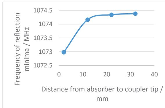
Figure 15: Frequency of the 2<sup>nd</sup> reflection minima as a function of absorber position.
