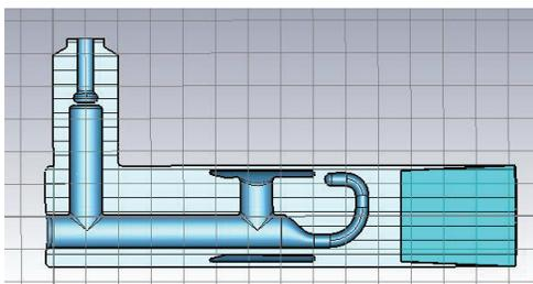
Figure 12: The DQW HOM coupler terminated into a 70 mm long conical SiC absorber with radii 31mm and 28 mm.
