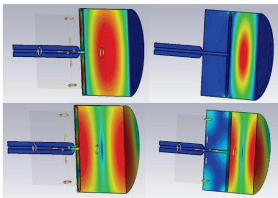
Figure 19: Manipulation of the TE<sub>111</sub> mode from 500MHz (left) to 812MHz (right) through use of the variable plate (Electric field top, magnetic field bottom).
