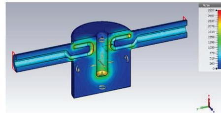
Figure 9: Electric field map at 400MHz for the RFD FPC test box. (Absolute magnitude, linear scale).
