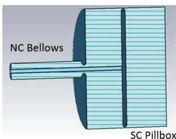
Figure 18: A basic model of a variable pillbox cavity. The section on the left contains the normal-conducting bellows, and no field. The section to the right is the superconducting region of high field where the couplers will be positioned.
