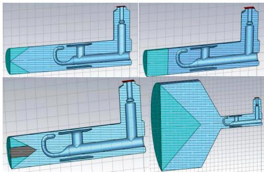
Figure 16: The four rejected designs for the DQW low power HOM test box. Inverted SiC cone (top left) straight block of SiC (top right), SiC cone in coaxial waveguide (bottom left), and tapered waveguide with SiC cone (bottom right).
