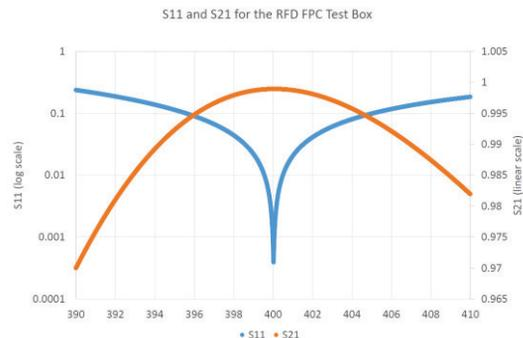
Figure 11:  $S_{11}$  and  $S_{21}$  for the RFD FPC test box over a 20MHz span centered on the operating frequency.
