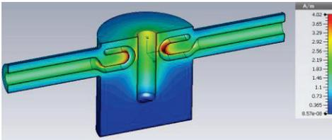
Figure 5: Magnetic field map at 400MHz for the DQW FPC test box. (Absolute magnitude, linear scale).
