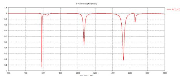
Figure 14: Reflections when the coupler is terminated in an open boundary.
