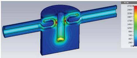
Figure 4: Electric field map at 400MHz for the DQW FPC test box. (Absolute magnitude, linear scale).
