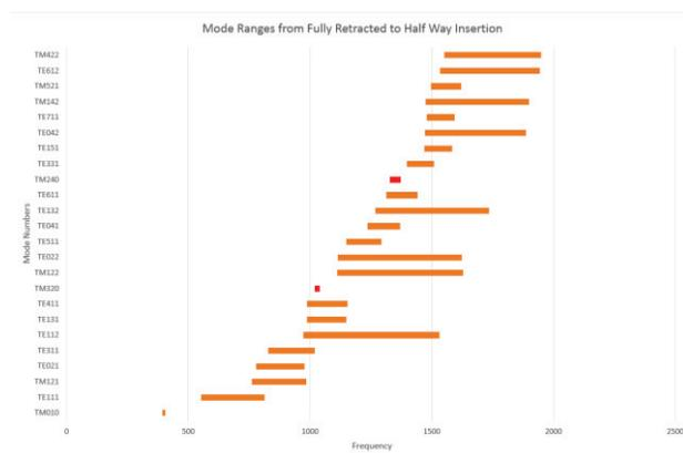
Figure 20: Plot of mode labels against frequency range in the variable pillbox cavity, from maximum length to half length.
