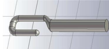
Figure 7: The RF dipole FPC hook.
