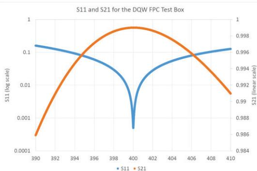
Figure 6: The reflection coefficient for the DQW FPC test box over a 20MHz span centered on the operating frequency.
