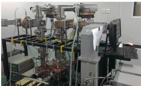
Figure 9 :Test bench for RF power coupler.
