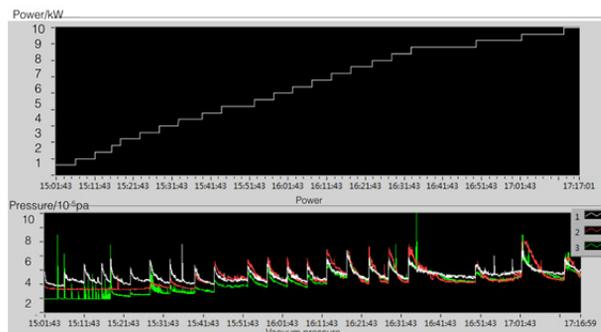
Figure 10: Records of RF power (upper) and vacuum pressure (lower) during conditioning.
