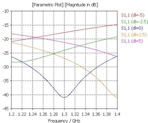
Figure 6:  $S_{11}$  vs. RF frequency with different  $dl$ .
