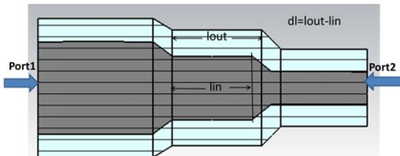
Figure 5: Model of a  $\lambda/4$  impedance transformer used for CST simulation.
