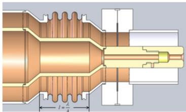
Figure 4: Bellows within the  $\lambda/4$  impedance transformer.
