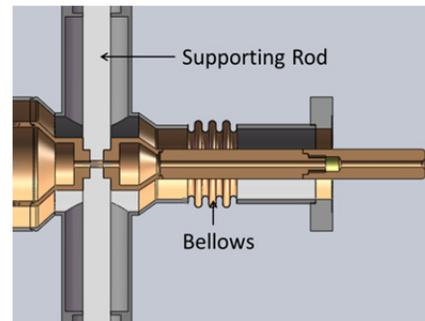
Figure 7: Bellows on 50Ω coaxial line.
