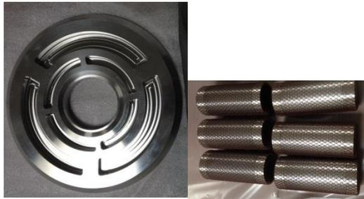
Figure 9: Flange (Left) and mandrel (Right) of the tube.
