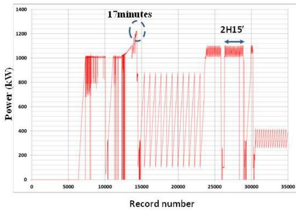
Figure 3: Power test on the HIPPI coupler.
