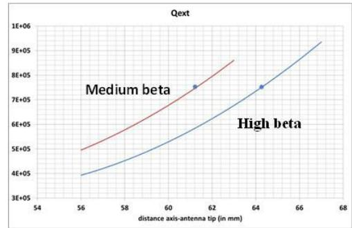
Figure 4: Simulation of the “antenna-cavity” coupling.
