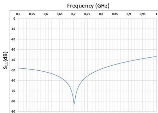
Figure 6: Return losses of the window.
