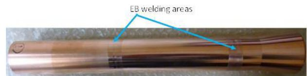
Figure 8: Antenna sample.
