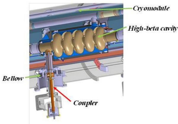
Figure 1: Coupler mounted on a high beta cavity.
