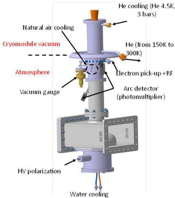
Figure 5: Interfaces and cooling circuits.
