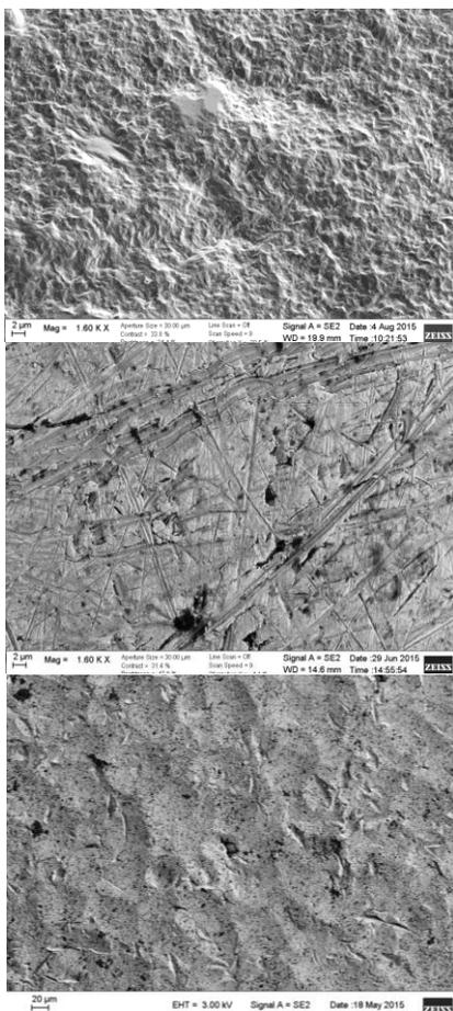
Figure 3: SEM photos of 150 μm thick copper plating: (top) bellow with no post processing, (middle) Mo wool polished bellow and (bottom) bead blasted coupon.
