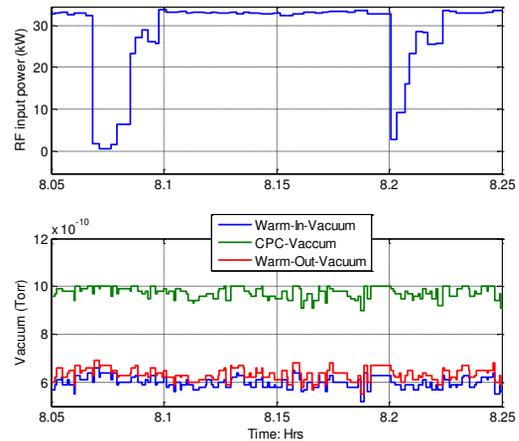
Figure 8: Data taken during RF processing of a pair of couplers with 30 kW pulses of 1 msec at 5 Hz. The top plot shows the power and the bottom plot the vacuum levels in the three coupler volumes (two warm sections and common cold section with connecting waveguide).
