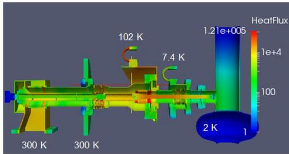
Figure 6: Simulation of the coupler heat flow given the measured/expected thermal intercept temperatures that are shown. The color map is of the heat flux ( $W/m^2$ ).
