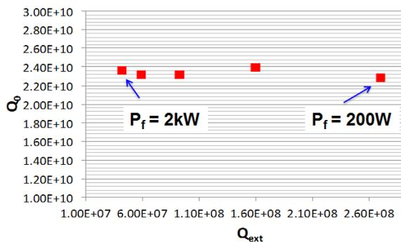
Figure 7: Measurements of the  $Q_o$  of a cavity at 15 MV/m at various input power levels ( $P_f$ ) achieved by changing the cavity external quality factor ( $Q_{ext}$ ) using the coupler antenna adjustment feature.
