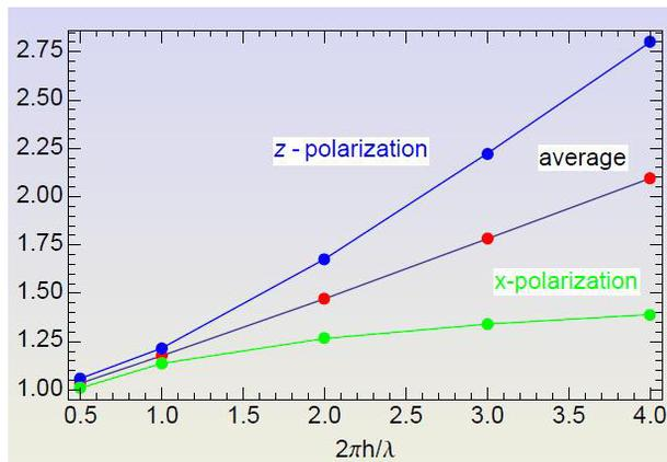
Figure 4: RF loss enhancement for sinusoidal surface variations with two H field polarizations.
