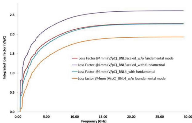
Figure 2: Integrated loss factors of the BNL4 cavity and the BNL3\_scale cavity, for the rms bunch length of 4 mm.
