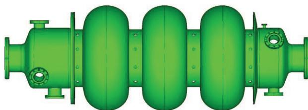
Figure 5: 3-cell prototype of the BNL4 cavity.
