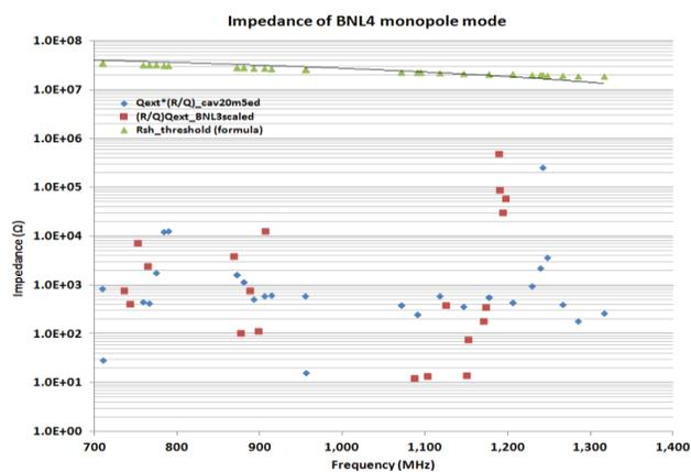
Figure 4: Impedances of monopole HOMs. eRHIC requirements (green triangles and the black line), BNL3 (blue diamond) and BNL4 (red square) cavities' monopole HOM damping capability.
