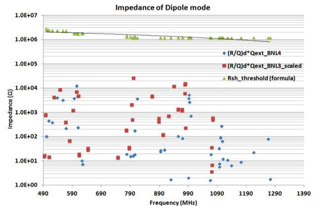
Figure 3: Impedances of dipole HOMs. eRHIC requirements (green triangles and the black line), BNL3 (blue diamond) and BNL4 (red square) cavities' dipole HOM damping capability.
