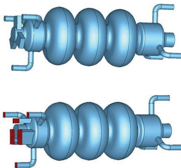
Figure 6: Two potential HOM damping schemes.
