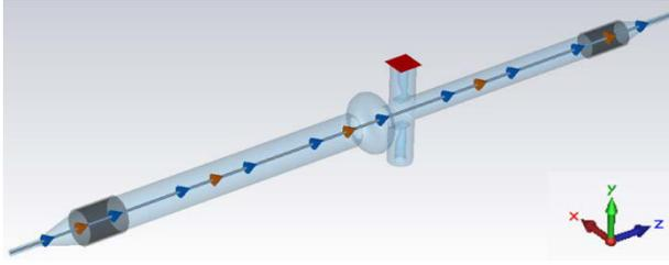
Figure 3: RF model used for wakefield and eigenmode simulations.
