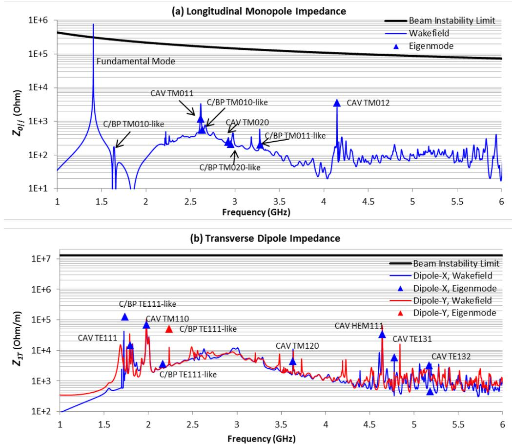
Figure 5: Monopole and dipole impedances calculated in the wakefield and eigenmode simulations. (a): longitudinal impedance for monopole modes, (b): transverse impedance for dipole modes. The resolution in results of the wakefield simulations is 200 kHz. CAV: cavity, C/BP: coupler and beam pipe.
