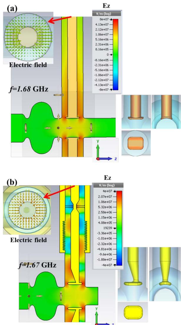
Figure 2: The first coupler mode with two different antennas calculated using the CST Eigenmode Solver. (a): initial design with the symmetric antenna, a TE<sub>11</sub>-like mode is trapped around coupler tip, (b): modified design with the asymmetric antenna to extract the previously trapped mode out by converting it to TEM mode. This mode can not propagate along the beam pipe so the beam pipe in the right side is reduced for the simulation in the modified design (b).
