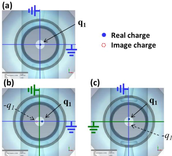
Figure 4: Beam offset and symmetry condition for different modes; (a): monopole, (b): dipole-x, where electric field is normal to y-z plane, (c): dipole-y, where electric field is normal to x-z plane. The ground symbols indicate conditions for symmetry planes; green: ‘electric boundary’ where electric fields are normal, blue: ‘magnetic boundary’ where magnetic fields are normal.
