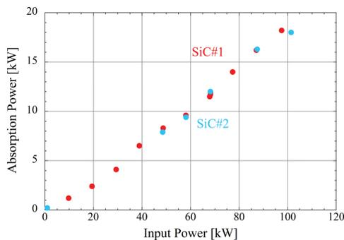
Figure 7: High power RF test results of the prototype of SiC dampers. The absorption powers of 18 kW were achieved by both dampers under the water flow rate of 15 L/min.
