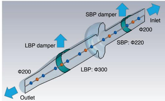
Figure 4: Calculation model of the SCC module with large beam pipes. The size of inlet and outlet beam pipes changed from 150 mm to 200 mm in diameter.
