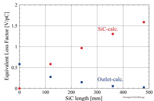
Figure 3: Equivalent loss factors of SiC damper (red) and the emitted out to the next cavity (blue). The length of 240 mm is suitable for the practical condition.
