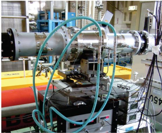
Figure 6: High power RF test stand with 509 MHz coaxial line for HOM damper of SCC module. The test stand consists of a klystron, a circulator, two dummy loads, a water cooling system for damper, thermometers and RF power meters.
