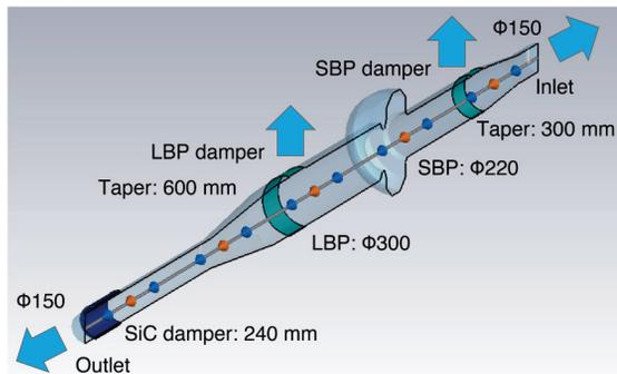
Figure 2: Calculation model of the SCC module. Bunched beam comes from inlet side. Monitors are set at SBP and LBP ferrite dampers, additional SiC damper and both ends of beam pipes (inlet and outlet)
