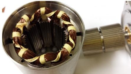
Figure 11: Phytron stepper motor internal windings after irradiation with dose  $5 \times 10^8$  Rad.
