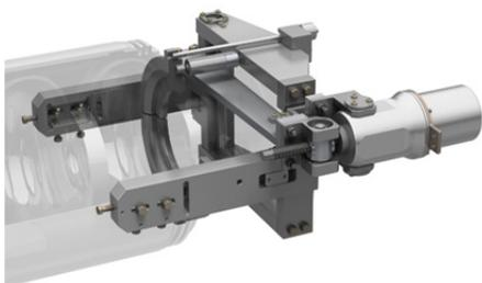
Figure 1: 3-D model of the LCLS II Tuner.
