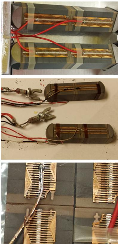
Figure 9: Top: sample A & B before irradiation test. Middle: sample A & B after 5\*10<sup>8</sup> Rad dose. Bottom: Central part of the two piezo-stacks (epoxy layer between two 10\*10\*18mm piezo): left- sample B (after 5\*10<sup>8</sup>Rad) and right - sample C.
