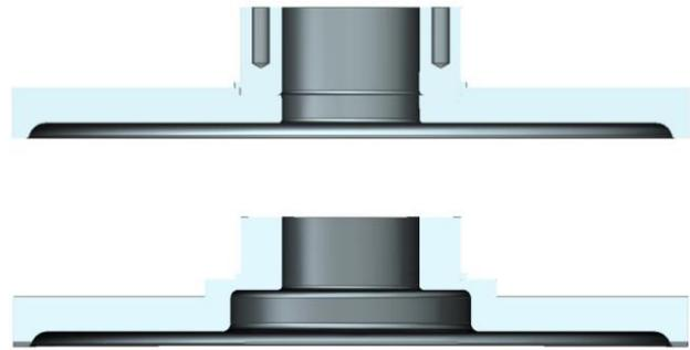
Figure 6: The original End Cap (top) and modified version (bottom).
