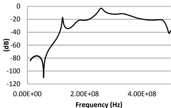
Figure 8: S21 feedback for BNL01 at a tuning displacement of 11.5mm, showing a notch frequency of 56.3 MHz.
