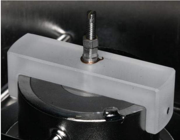
Figure 5: Sapphire Bridge positioned on the Filter Assembly in BNL03. The damper is shown in its un-tuned state.
