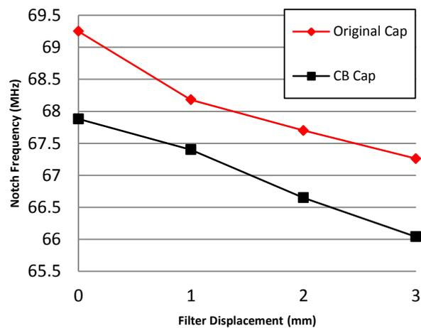
Figure 7: Comparison of original and counter-bored (CB) cap for BNL03 tuning.
