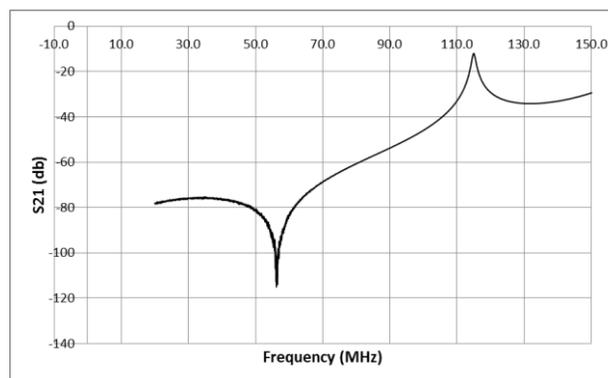
Figure 4: Network analyser output from tuning process of the prototype [1]. Target is first notch being set to 56.3 MHz.
