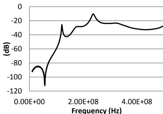
Figure 10: S21 feedback for BNL03 at a tuning displacement of 12mm, showing a frequency of 57.0 MHz.
