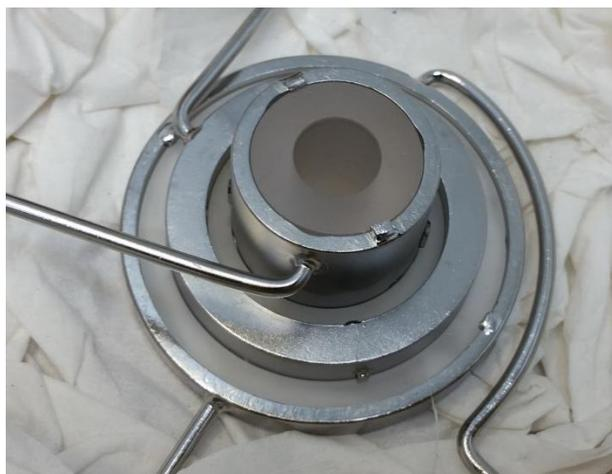
Figure 2: Filter Assembly, showing the Nb ‘stoppers’ and Inductor Rods.
