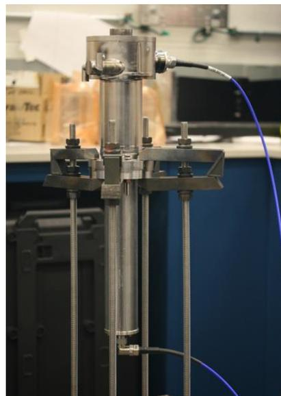
Figure 3: Tuning setup for BNL01.
