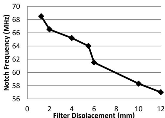
Figure 9: Notch frequencies of BNL03 while tuning.
