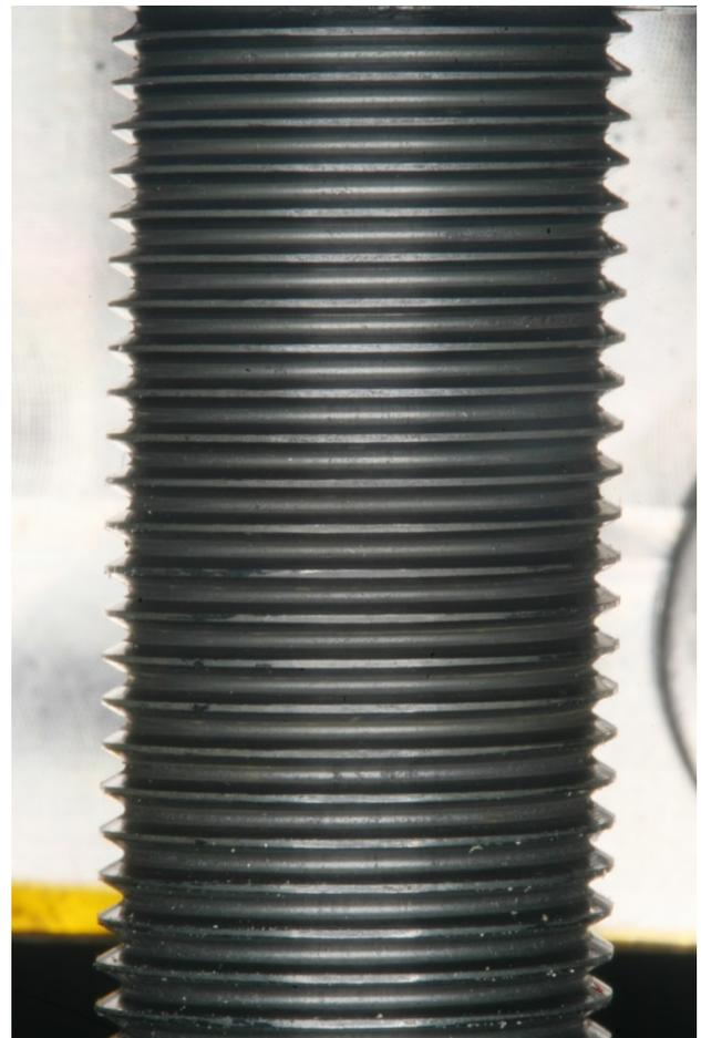
Figure 6: Motor spindle after initial test runs, showing no damage or loss of lubrication.
