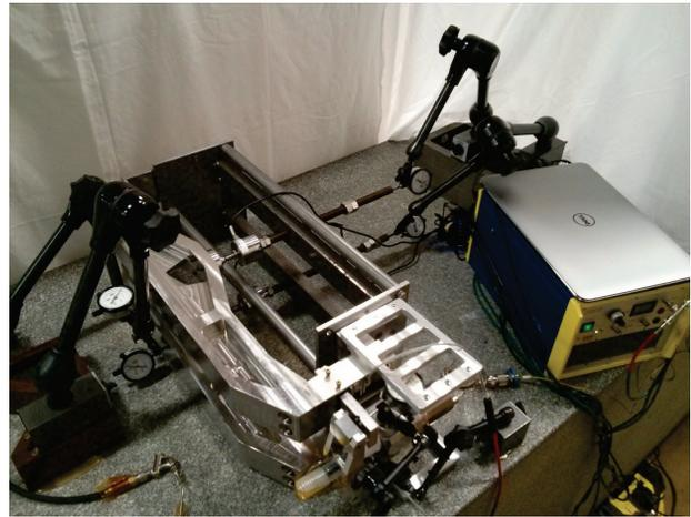
Figure 4: Tuner mounted on a test stand for initial measurements at room temperature.
