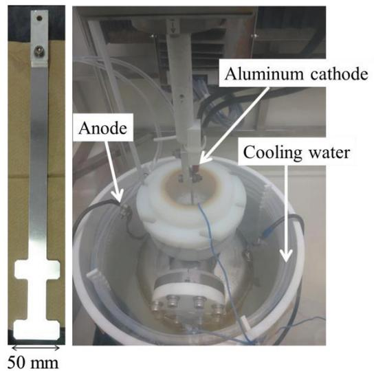
Figure 8: Vertical electro-polishing of the SRF gun #1.
