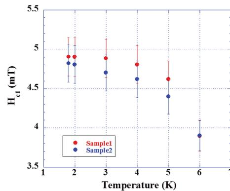
Figure 4: Lower critical magnetic field (Hc1) of LiTi<sub>2</sub>O<sub>4</sub>. Sample 1 is before forming bi-alkali layer. Sample 2 is after forming bi-alkali layer.
