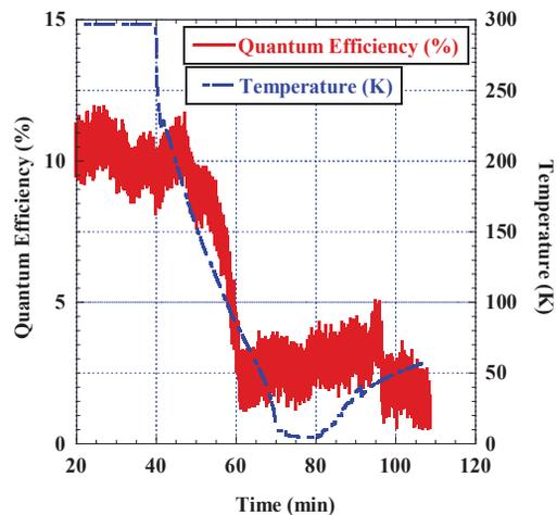
Figure 5: One example of the cooling test of the photocathode in DC gun.
