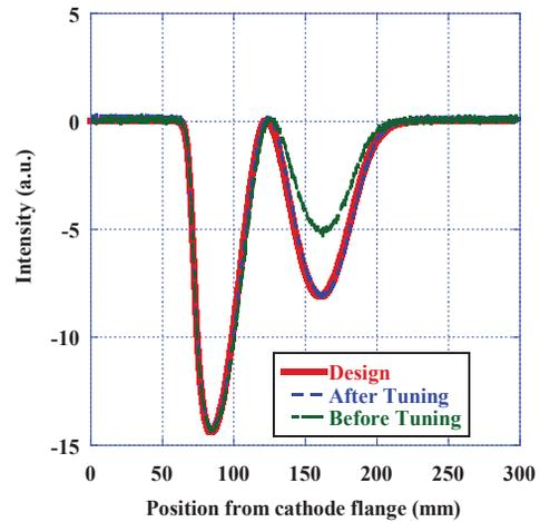
Figure 7: Electric filed distribution of the SRF gun #1.
