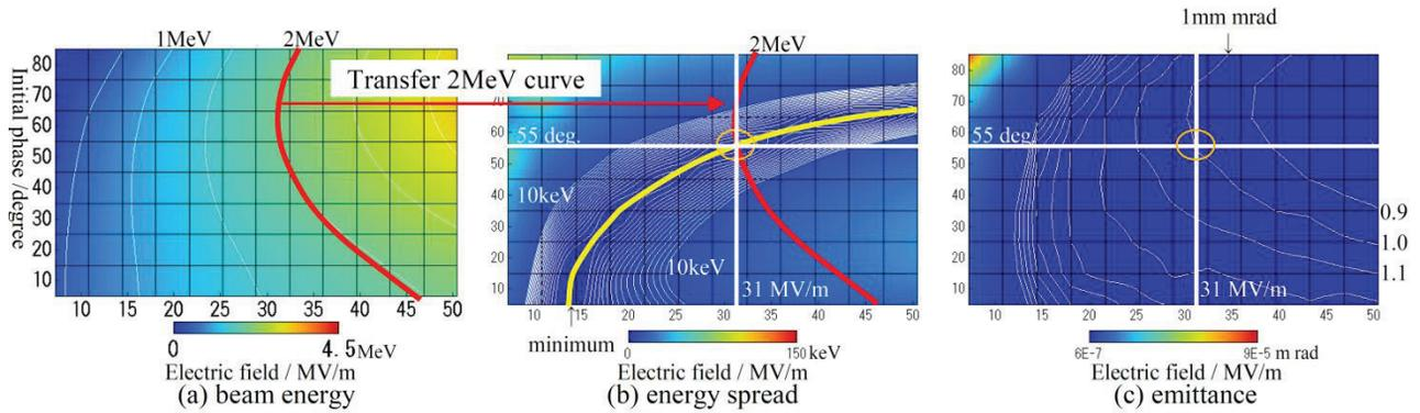
Figure 2: Contour map of beam specifications at cavity exit.
