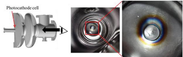
Figure 11: Color change of the cathode cell.
