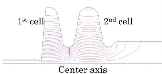
Figure 3: RF electric field analysis by SUPERFISH.
