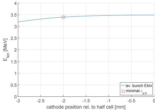
Figure 3: Diagram of kinetic energy at the gun’s exit versus the position of the retracted cathode tip, zero being no retraction at all. The highlighted spot corresponds to a minimal emittance at 2.8m from cathode as found by the scan shown in figure 4.
