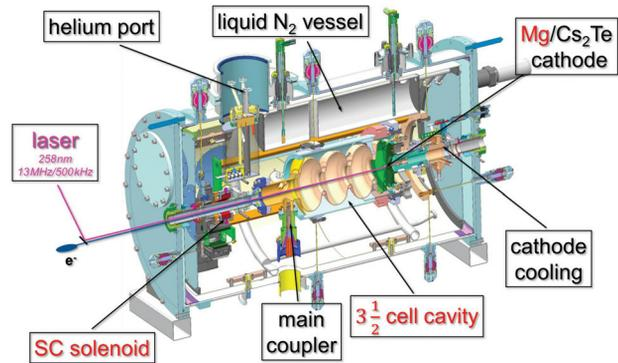
Figure 1: Overview of the design of the ELBE SRF Gun II.
