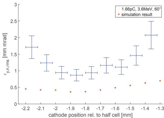
Figure 10: Result of a first test scan of the transverse emittance versus the cathode position performed with a low charge bunch.
