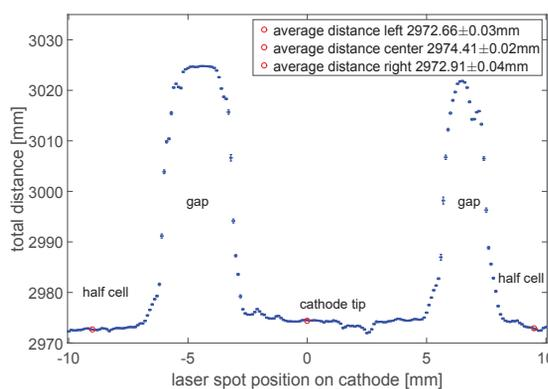
Figure 8: Result of a cathode localization measurement. The distance values left and right of the center represent the distance of the measuring device to the half cell around the cathode, while the inner part represents the distance to the cathode’s front tip. The gaps in between are less wide in reality (> 1 mm), but cause a much larger signal here due to the size of the scanning laser’s spot at this distance .
