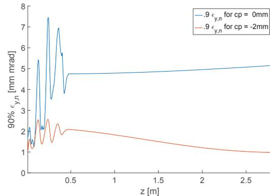
Figure 5: The evolution of the core emittance for a 250 pC bunch along the beam line with and without RF focusing.
