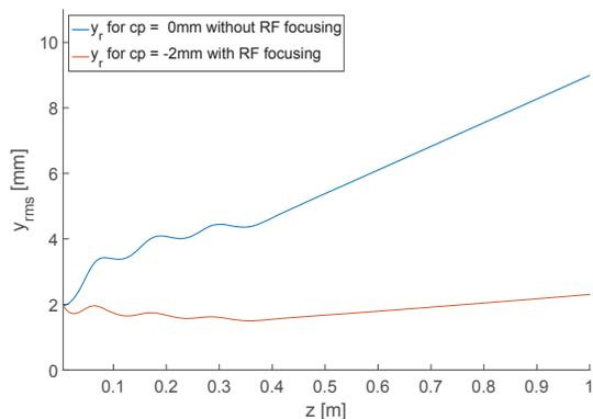
Figure 6: Comparison of the development of the beam radius for the first meter along the beam line for a 250 pC bunch with and without RF focusing.
