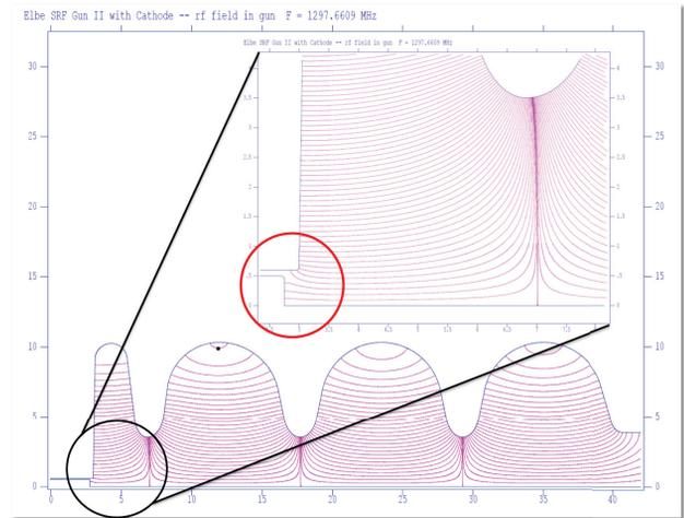
Figure 2: Example of the transverse electrical field lines affecting the cathode tip. In the indicated area the effect of RF focusing becomes visible, as the field representations indicate the additional focus towards the central gun axis for a retracted cathode.
