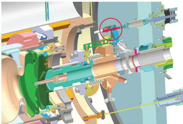
Figure 7: CAD image for the cathode cooler, half cell of the resonator and the cathode tuner inside the gun cryostat. The indicated mechanism connects the cathode holder to a gear outside the cryostat, making it possible to move the cathode tip in and out of the resonator during operation.
