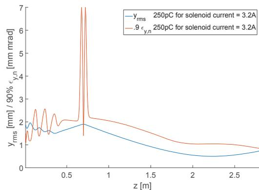
Figure 11: Combination of the impact of RF focusing and the SC solenoid (at about  $z = 70$  cm) on the core emittance and the transverse extension of the beam.
