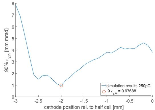
Figure 4: Scan of the transverse core emittance at the second screen ( $z = 2.8$  m) station for different cathode positions behind the back plane of the resonator.
