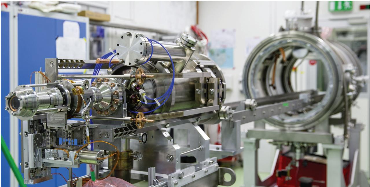
Figure 9: Photograph taken of the cavity string including the SC solenoid and its horizontal and vertical stepper before insertion into the cryostat in the right part of the picture.
