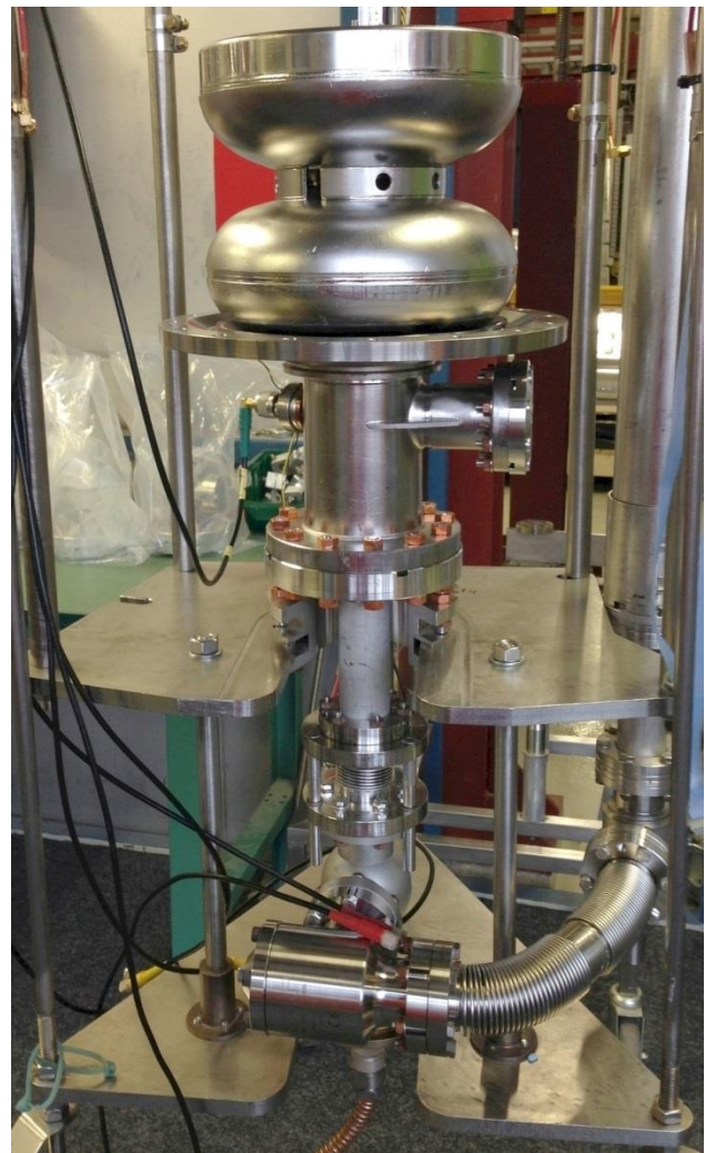
Figure 2: SRF gun cavity in a vertical test cryostat insert at DESY, Hamburg.
