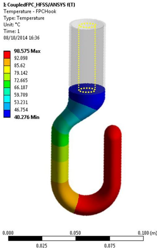
Figure 3: Temperature distribution in the FPC hook for nominal deflecting voltage from HFSS/ANSYS simulations. The dotted yellow lines represent the cooling channel opened in the coupler stem.
