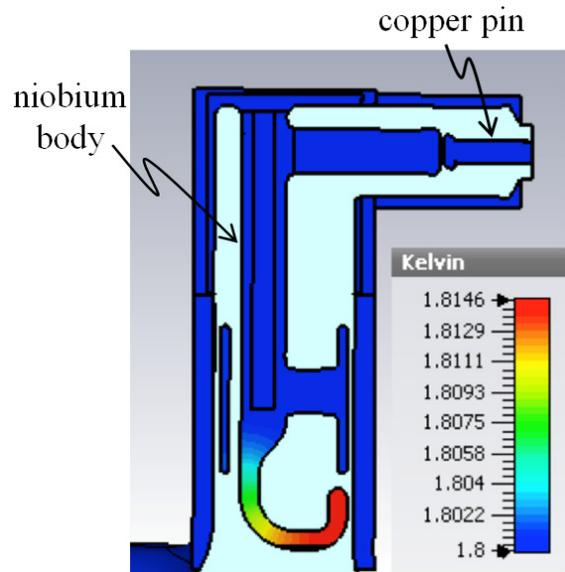
Figure 5: Temperature distribution in the HOM filter for fundamental mode and deflecting voltage of 1 MV (CST simulations).
