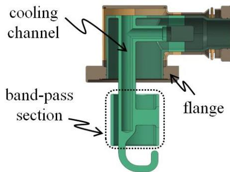
Figure 4: CAD model for the HOM filter showing the cooling channel.
