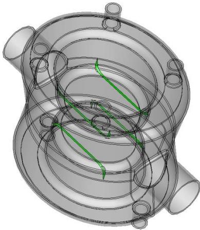
Figure 3: Shell model with an ideal stiffener: zero-displacement was applied to the interfaces where the stiffener was welded to the cavity central plates (highlighted in green).
