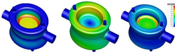
Figure 1: Electric (left) and magnetic (center) field distributions for the fundamental mode of the PoP DQWCC and corresponding Lorentz force density (right) [CST simulation].
