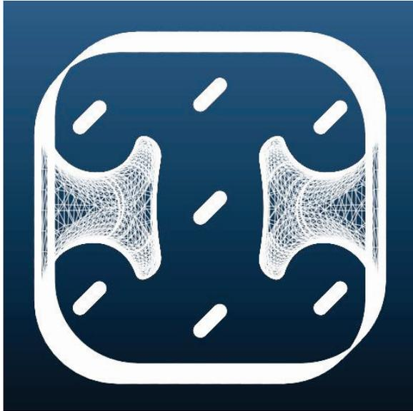
Figure 9: Possible cathode configuration with seven cathode rods of niobium.
