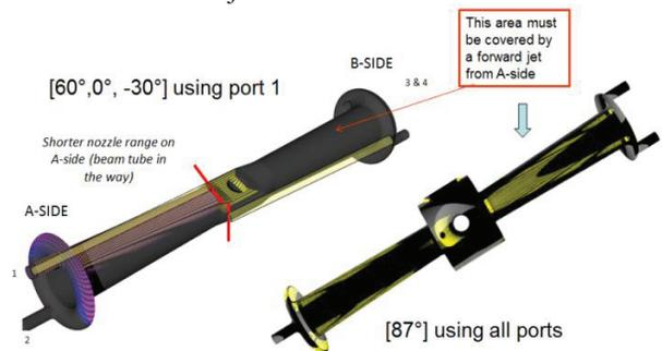
Figure 6: Improvement of cone coverage with a 87° jet.
