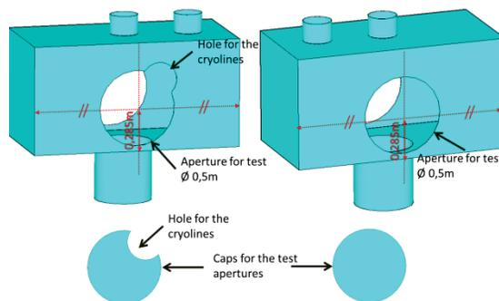
Figure 16: Magnetic shields apertures and caps.
