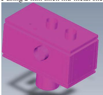
Figure 15: Sathori magnetic shield design.
