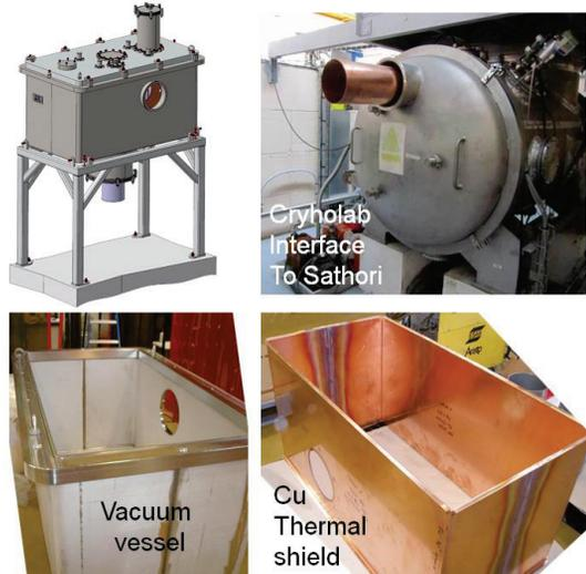
Figure 14: Manufacturing of Sathori components.
