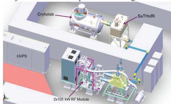
Figure 12: Cryholab-Sathori layout in Saclay test area.
