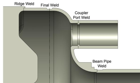
Figure 3: Details of the weld preparations for the cavity welds. The final weld will require a full penetration weld using a TIG welder from the outside of the cavity.
