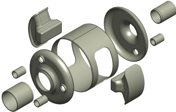
Figure 2: An exploded view of the individual Niobium components that will be welded together to form the cavity.
