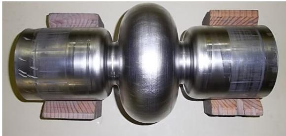
Figure 4: Niobium tube just after hydroforming.
