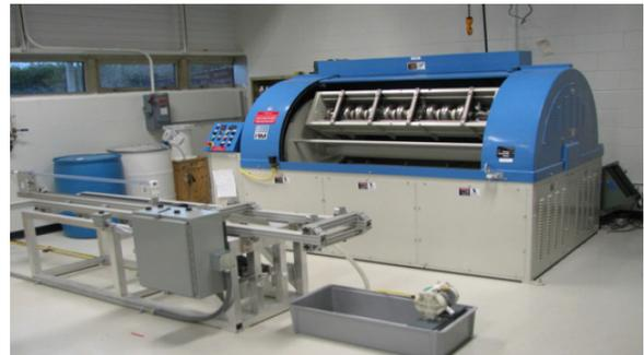
Figure 7: Barrel polishing machine<sup>[8]</sup>.
