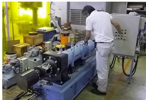
Figure 3: Hydroforming machine (Final hydraulic pressure: 25 MPa).
