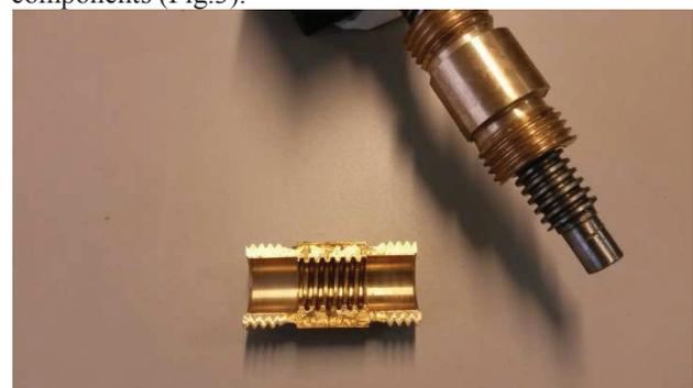
Figure 3: CTM spindle and gear box with early wear out.
