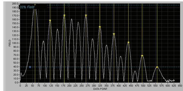
Figure 4a): Example for TM011 field distribution- asymmetrical cavity (maximum at first cell).
