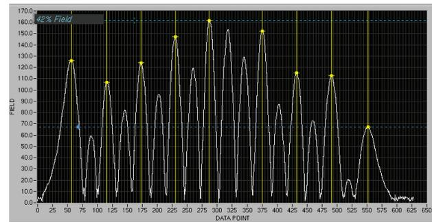
Figure 4b): Example for TM011 field distribution- symmetrical cavity (Maximum at middle cell).
