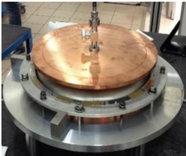
Figure 3: RF measurements system (on half cell).
