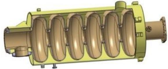
Figure 1: Medium beta elliptical cavity with helium tank.
