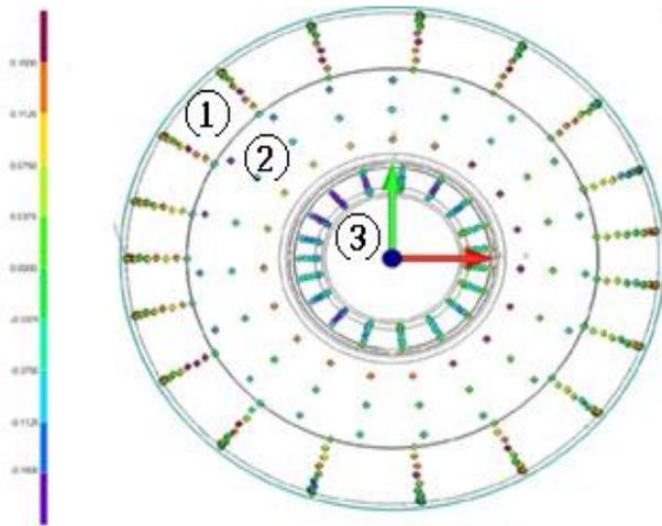
Figure 6: 3D CMM result on a central half cell, red +0.15mm, purple -0.15mm.
