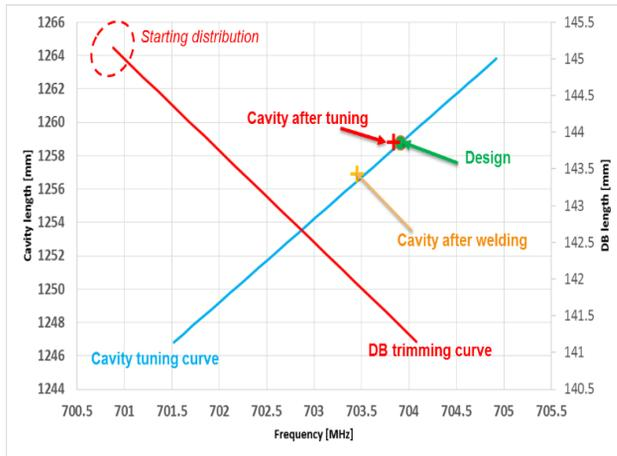
Figure 14: Dumbbells and cavity length vs. frequency plot. Red line represents the dumbbell trimming curve, blue line the cavity tuning curve, the yellow cross represents the expected value for the 1<sup>st</sup> manufactured cavity just after welding, red cross after tuning and the green dot the design value.
