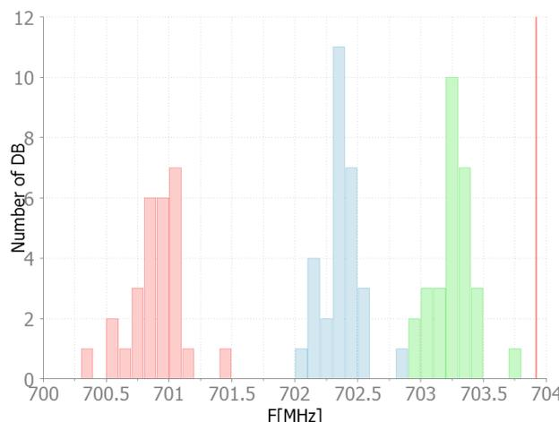
Figure 13: Dumbbells  $\pi$ -mode frequency evolution from welding (red), trimming (blue) and trimming+welding shrinkage (green). The vertical red line corresponds to the target value.
