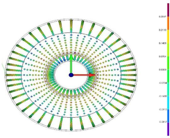
Figure 11: Dumbbells upper cell 3D measure, red +0.28mm, purple -0.28mm.
