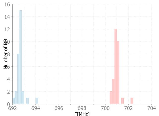
Figure 9: Dumbbells RF measurements for 0-mode (blue) and  $\pi$ -mode (red). Each bin has 0.2MHz width.
