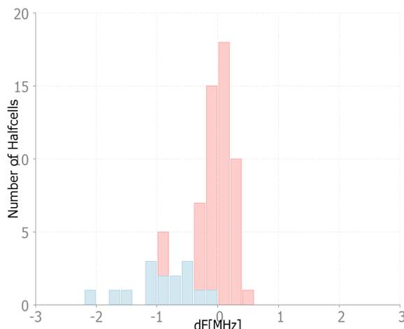
Figure 4: 0-mode frequency shift between design value and measure on central halfcells (red) and end group (blue), each bin has 0.2MHz width.
