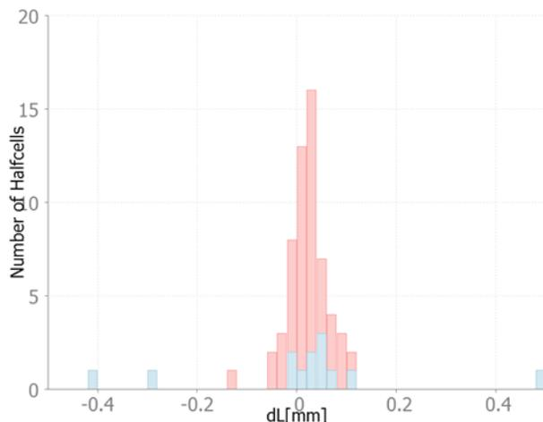
Figure 5: Length difference between simulated and measured values on central group (red) and end group (blue) halfcells, each bin has 0.02mm width.
