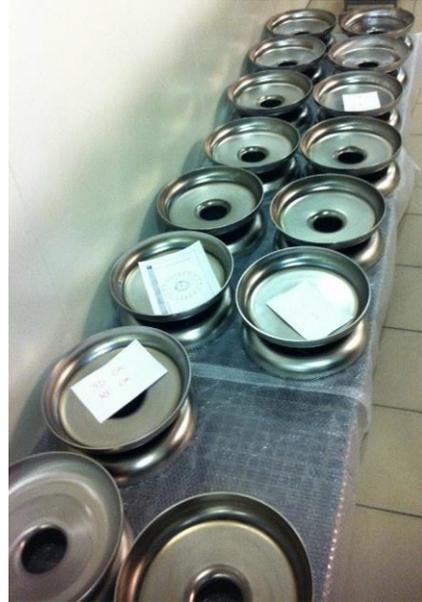
Figure 8: Dumbbells after welding in the control area.
