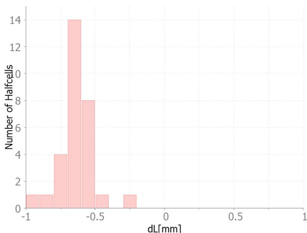
Figure 10: Dumbbells length difference with design value, each bin has 0.1mm width. Measure performed after welding and reshaping.
