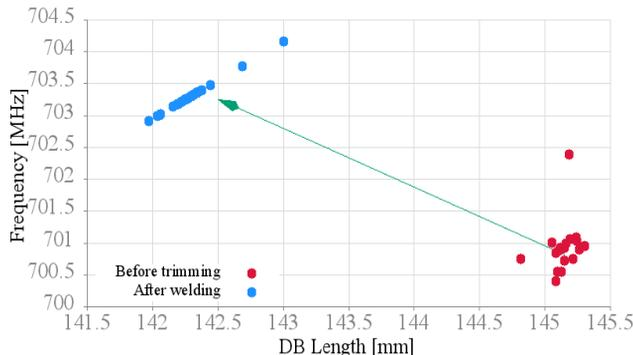
Figure 12: Dumbbells length and  $\pi$ -mode frequency before trimming as measured (red dots) and computed values with trim and weld shrinkage (blue dots).
