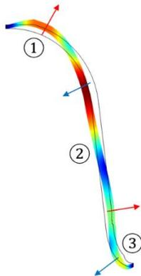
Figure 7: Scheme of average deformation observed on central half cell (not in scale).
