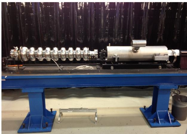
Figure 2: Assembly and alignment fixture.
