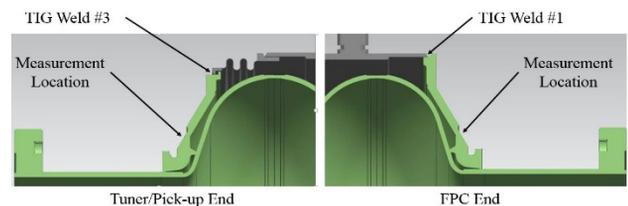
Figure 9: Temperature measurement locations.
