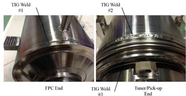
Figure 8: Close-up view of finished TIG welds.
