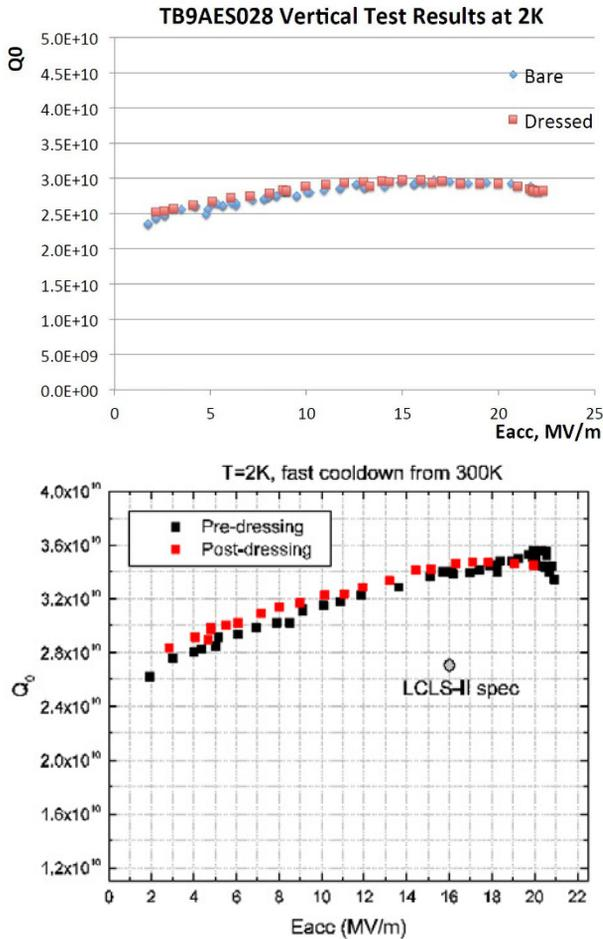
Figure 10: Q vs. E plots for a bare and dressed cavity.
