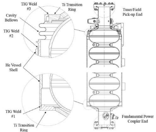
Figure 1: Section view of dressed cavity showing the weld joint geometry.
