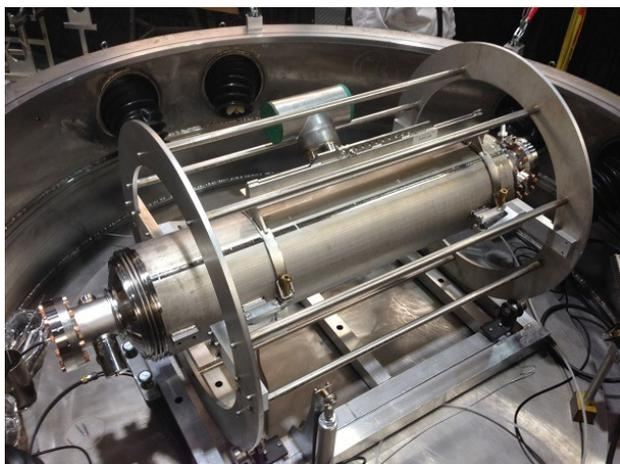
Figure 3: Cavity installed in rotation fixture.
