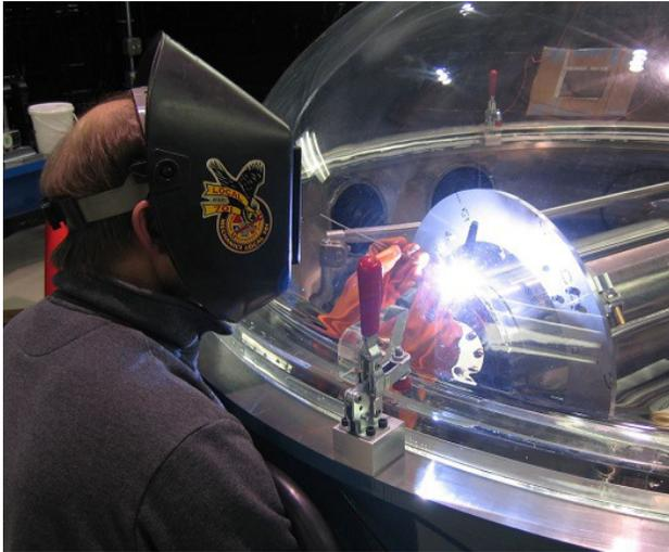
Figure 6: Welding in the glove box.
