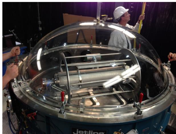
Figure 4: Cavity installed in glove box.
