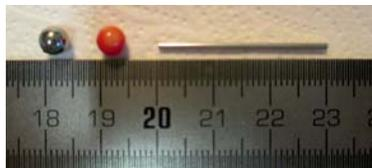
Figure 5: Perturbing objects used. From left to right: metallic sphere, dielectric sphere, cylindrical metallic needle.
