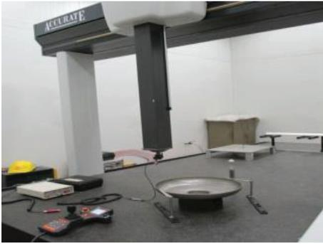
Figure 21: CMM measurement of half-cell.
