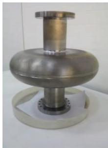
Figure 24: Single cell elliptical cavity after EBW.
