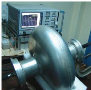
Figure 12: Single cell Aluminium prototype cavity.
