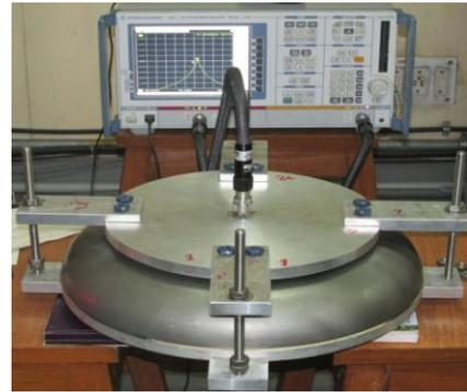
Figure 25: VNA measurement of niobium half-cell.
