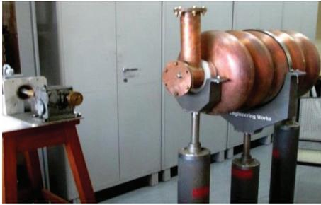
Figure 14: 5-cell copper prototype cavity.
