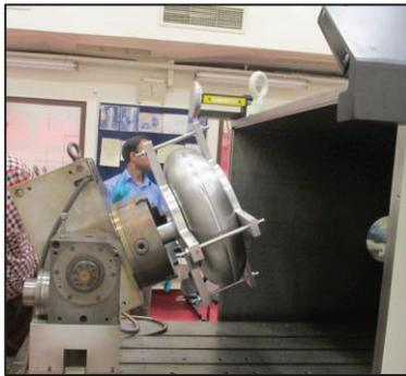
Figure 23: Cavity half cells being put inside EBW machine for equator welding at IUAC, New Delhi.
