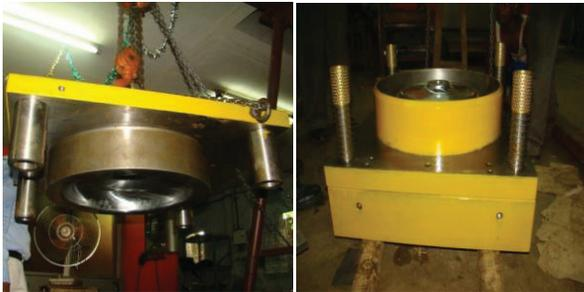
Figure 11: Die Punch Assembly for the cavity.
