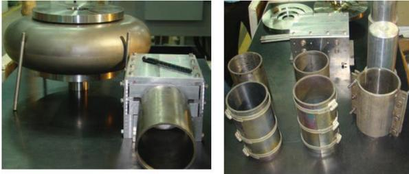
Figure 22: Niobium half cells and beam pipes with fixtures developed for Electron Beam Welding.
