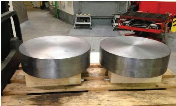
Figure 2: CBMM Large Grain ingots at Heraeus in preparation for the slicing process.
