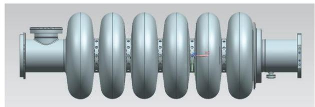
Figure 1: Sketch of the “Type 2” medium beta cavity.
