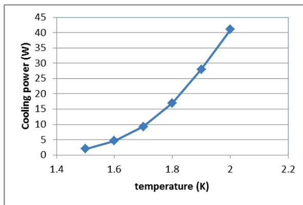
Figure 6: Cooling power vs. temperature for LASA cryogenic sub-cooling system.
