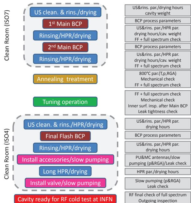
Figure 4: ESS prototype cavities treatment flow and recorded parameters.
