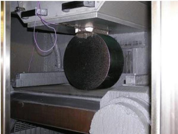
Figure 3: Wire sawing process at Heraeus for a 300 mm diameter ingot.
