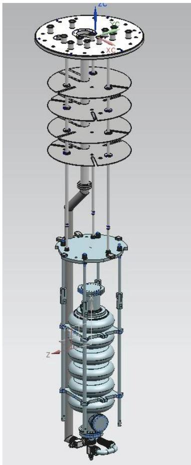
Figure 5: Model of the new cold insert for the ESS cavities test.
