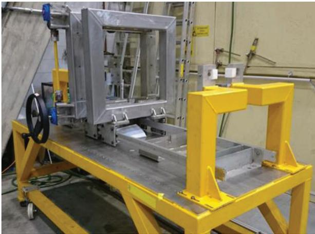
Figure 8: The LASA cavity tuning machine.
