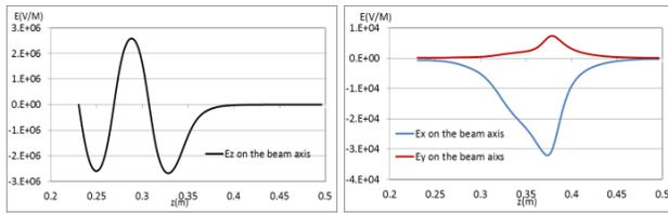
Figure 5: The accelerating field longitudinal (left) and transverse (right) components on the beam axis in the downstream HOM/FPC endgroup and its neighbouring 3 cells.
