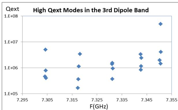
Figure 9: The high  $Q_{\text{ext}}$  modes damping in the 3<sup>rd</sup> dipole band in a 3.9 GHz 4-cavity chain.
