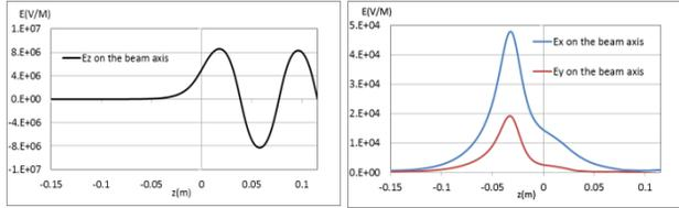
Figure 4: The accelerating field longitudinal (left) and transverse (right) components on the beam axis in the upstream HOM endgroup and its neighbouring 3 cells.
