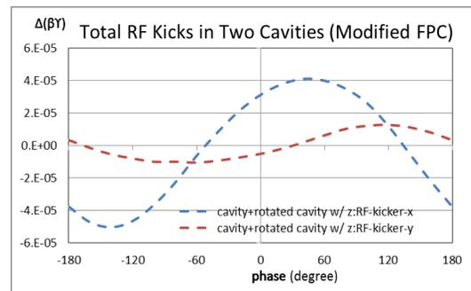
Figure 8: Cavity and rotated cavity arrangement (up) and the two cavities RF kicks (down).
