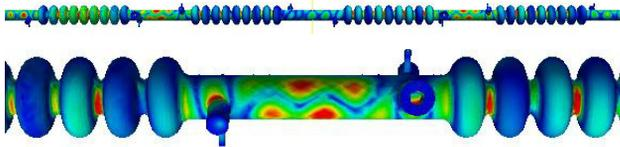
Figure 10: The first trapped mode around 7.35 GHz in a 3.9 GHz 4-cavity chain (top) and beampipe (bottom).
