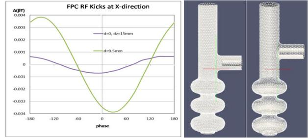
Figure 7: The FPC RF kicks in the current and proposed designs. d is the distance between the antenna tip and the beampipe wall.
