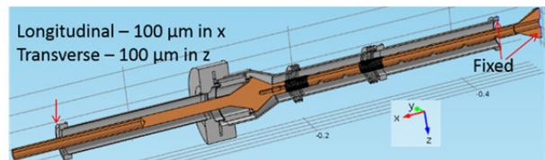
Figure 6: COMSOL solid model and mechanical boundary conditions.
