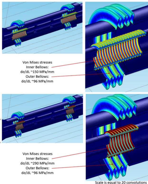
Figure 8: Von Mises stresses for original (upper) and modified (lower) couplers for longitudinal deformations.
