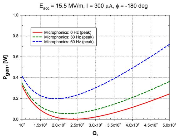
Figure 11: Input RF power required by the LCLS-II 3.9 GHz cavity with microphonics.
