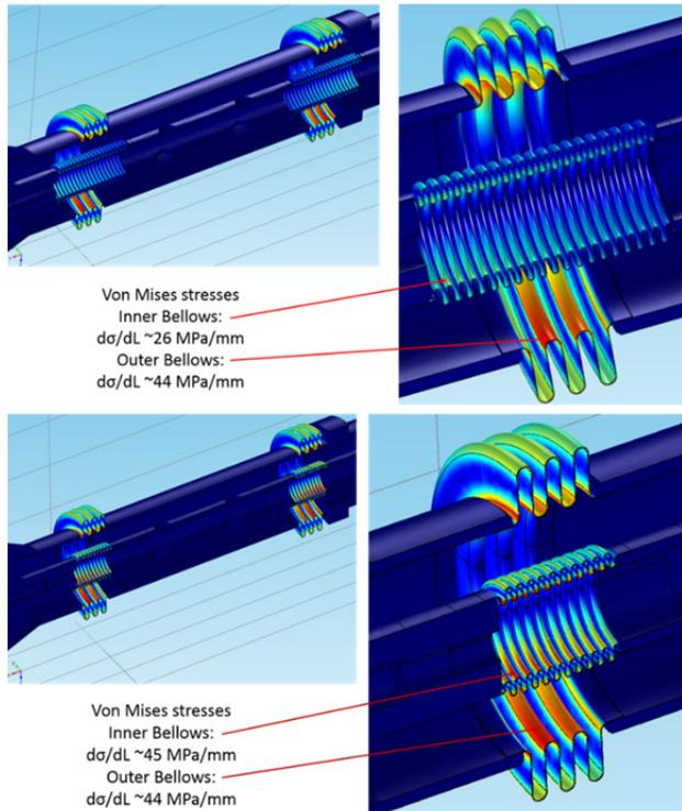
Figure 7: Von Mises stresses for original (upper) and modified (lower) couplers for transverse deformations.
