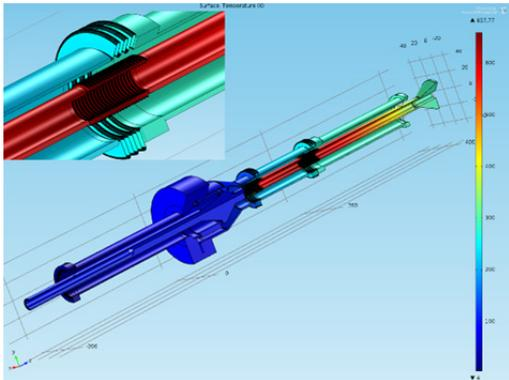
Figure 3: Temperature map in the TTF3 coupler with LCLS-II parameters. Max. Temperature is ~658 K.
