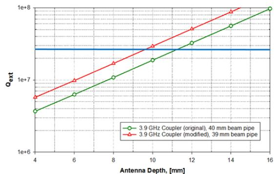
Figure 9: Coupler  $Q_{ext}$  versus antenna depth.
