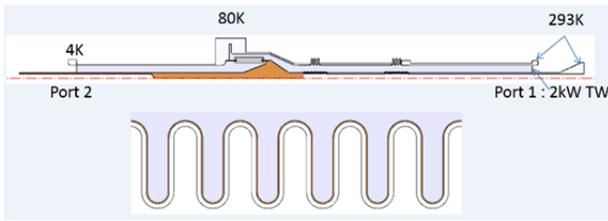
Figure 2: COMSOL thermal analysis model.
