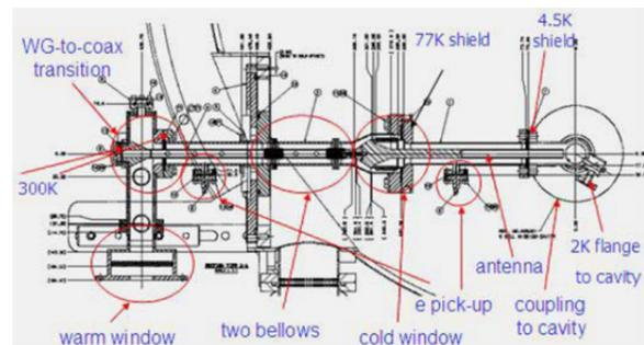
Figure 1: The 3.9 GHz power coupler developed at Fermilab.
