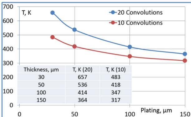
Figure 4: Maximum coupler surface temperature versus copper plating thickness and number of convolutions.
