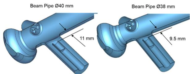
Figure 10: Antenna modification.
