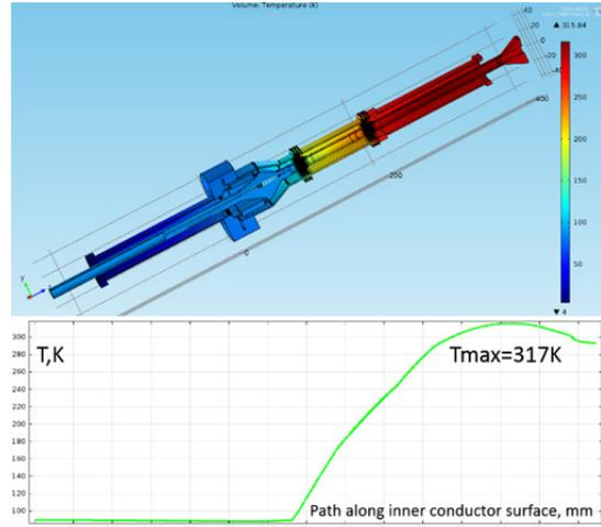
Figure 5: Temperature distribution along the coupler (up) and along the surface of the inner conductor (down) for modified coupler design.
