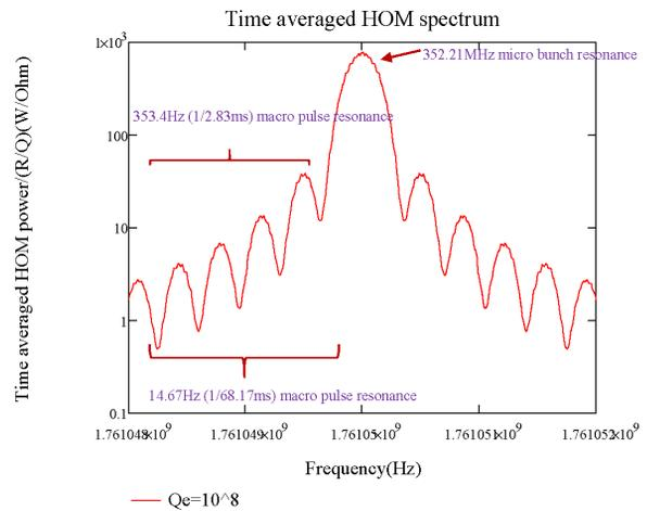
Figure 4: Time average power/  $(R/Q)$  at  $Q_e=10^8$  in one period of  $T_m$ .
