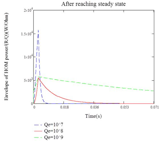
Figure 3: Normalized HOM power at  $f=1.76105$  GHz ( $5 \cdot 352.21$  MHz) between the macro-pulses in steady state at different  $Q_e$ .
