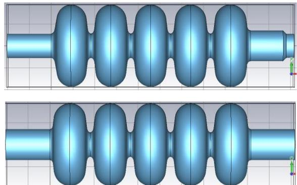
Figure 13: The profile of  $\beta=0.86$  cavity. (The up one is design 1. The bottom one is design 2.)
