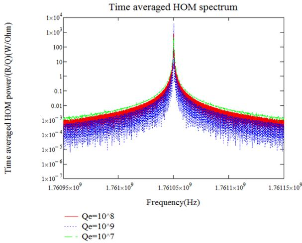
Figure 5: Time average power/ ( $R/Q$ ) at different  $Q_e$  in one period of  $T_m$  (span: 0.2 MHz).
