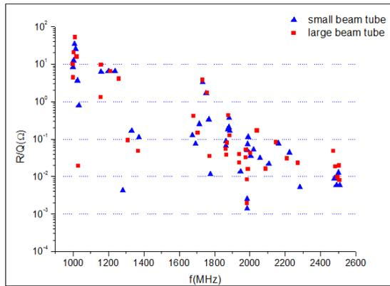
Figure 10:  $R/Q$  for dipole modes.
