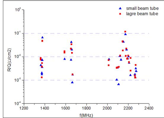
Figure 11:  $R/Q$  for quadrupole modes.
