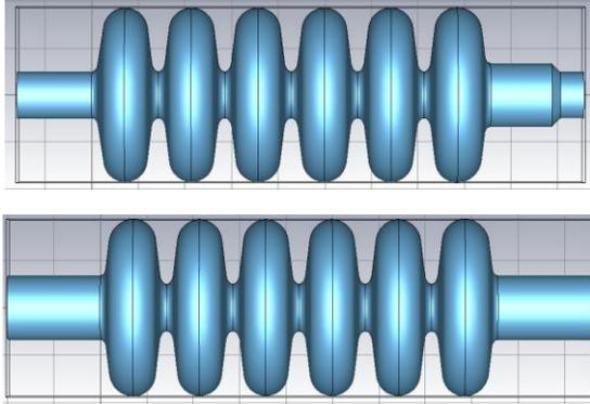
Figure 8: The profiles of two type cavities. (The upper one is design 1 with small beam tube. The bottom one is design 2 with large beam tube.)
