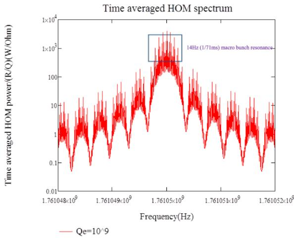
Figure 6: The normalized HOM power from the beam time structure of ESS around 1761.05 MHz at  $Q_e = 10^9$ .
