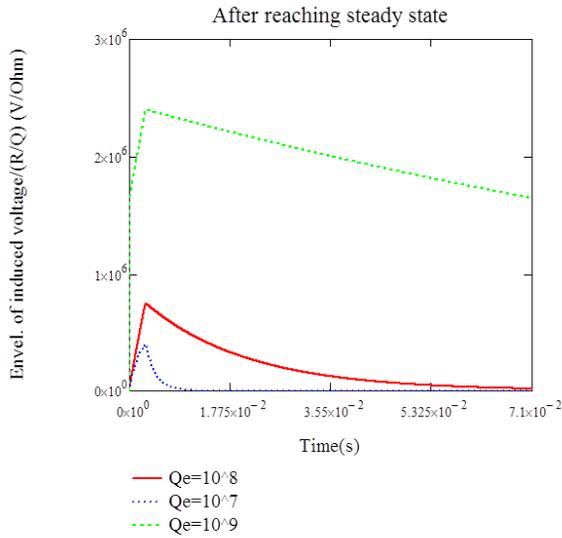
Figure 2: Normalized induced voltage /  $(R/Q)$  at  $f=1.76105$  GHz ( $5 \cdot 352.21$  MHz) between the macro-pulses in steady state at different  $Q_e$ .
