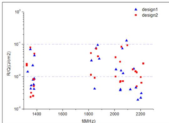
Figure 16:  $R/Q$  for quadrupole modes.
