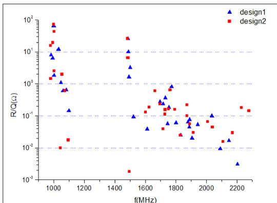
Figure 15:  $R/Q$  for dipole modes.
