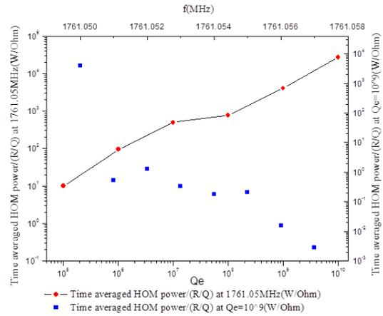
Figure 7: HOM power dependencies on the  $Q_e$  at micro-bunch resonance.
