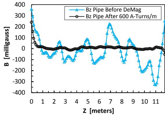
Figure 3: Field measured before and after demagnetization of the carbon steel vacuum vessel (Courtesy of A.C. Crawford).
