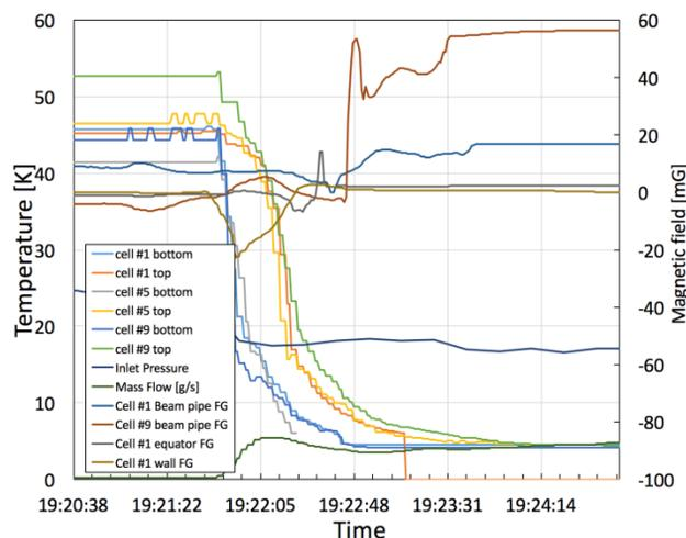
Figure 5: A small thermal current and high thermal gradient between the top and bottom of the cavity successfully expelled the remaining magnetic flux in the cavity during a fast cryogenic cool down [22].
