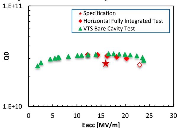
Figure 6: The  $Q_0$  of a horizontally tested fully integrated cavity is compared to its  $Q_0$  measured in vertical test. The empty diamond represents an estimated  $Q_0$  value at 23 MV/m when cavity is operated below quench field [22].
