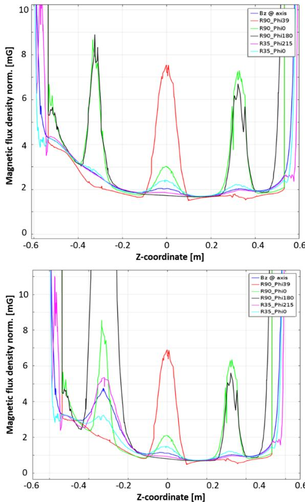
Figure 1: Effect of the magnetic tuner support bearing. Upper figure represents a nonmagnetic tuner bars. Lower figure represents a magnetic tuner bars [18] (Courtesy of I. Terechkine).
