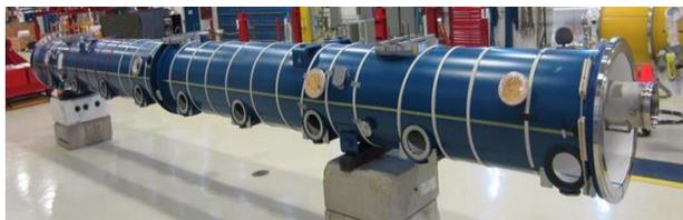
Figure 2: A prototype demagnetization coil wrapped around a LCLS-2 type vacuum vessel [19].
