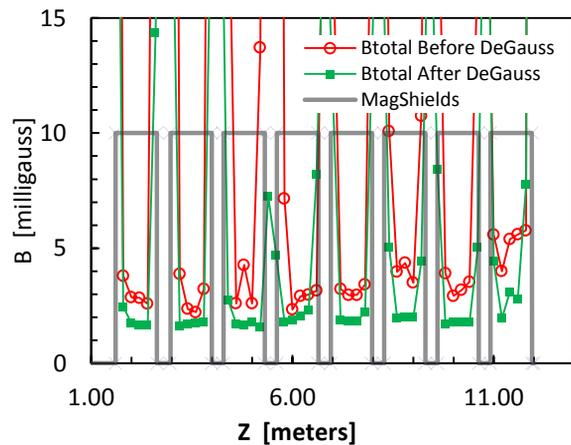
Figure 4: The Magnetic field at the shielding center showing the reduction of the cavity edge field (upper plot) and zoomed plot (lower plot) showing the reduction of the cavity center field after the in-situ demagnetization of a mock-up cryomodule (Courtesy of A.C. Crawford).
