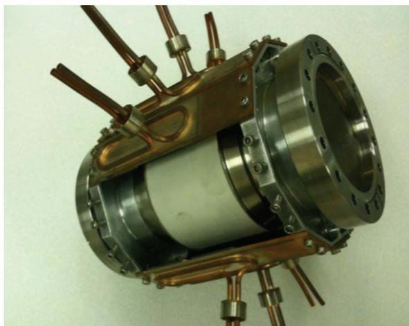
Figure 2: HOM absorber for the ECX cavity at BNL. The absorption of the microwaves is provided by ferrites. To shield them from the beam (which could charge-up the tiles) and to prevent contamination of the cavity (by ferrite particles and chips) a ceramic break is inserted.
