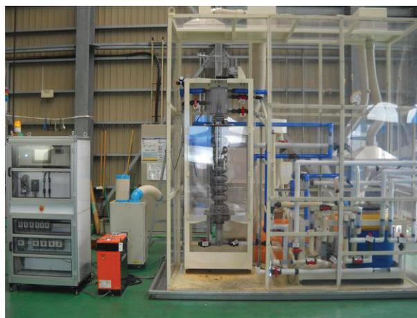
Figure 2: VEP setup for 9-cell cavity.
