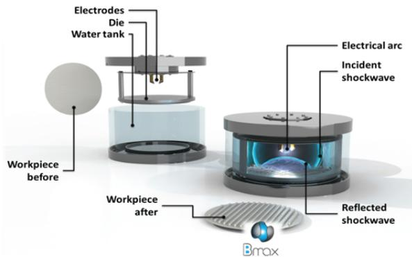
Figure 4: Electrohydraulic forming principle [8].
