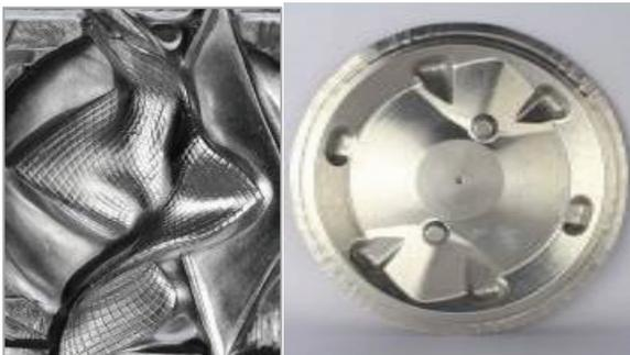
Figure 5: Example of Electro-Hydro Formed parts.
