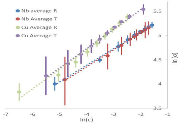
Figure 7: True stress vs true strain in log – log scale for Nb and Cu plates. The slopes of the curves determine the strain hardening exponent.
