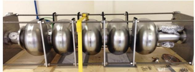
Figure 1: SPL 704 MHz elliptical cavity.
