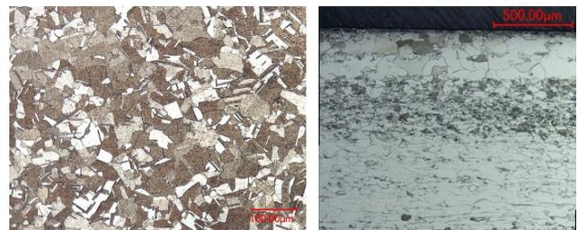
Figure 6: Metallographies of a copper plate (left) and a niobium plate (right) showing uniform equiaxed grains for the copper and slightly elongated grains in the core for the niobium plate.
