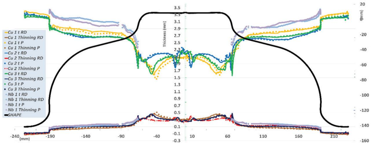
Figure 12: Final shapes of OFE copper half-cells thickness and thinning  $\epsilon_3$  distributions in sheet rolling and perpendicular direction.
