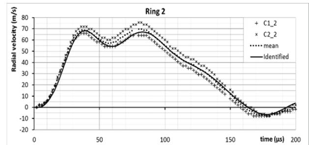
Figure 8: Measured ring expansion velocities (dots) and identified curves (lines).
