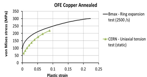
Figure 9: Stress-strain relation comparison for OFE copper between static and dynamic conditions.
