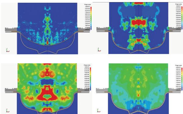
Figure 10: 2D-axisymmetric EHF simulations of a copper cavity using four different EHF discharges.
