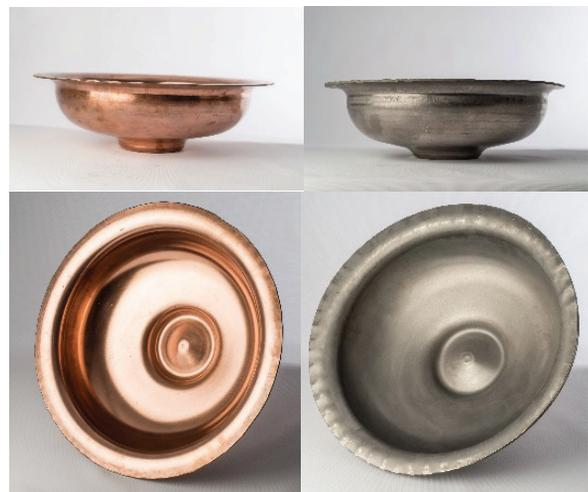
Figure 11: Half-cells in copper and niobium by EHF.
