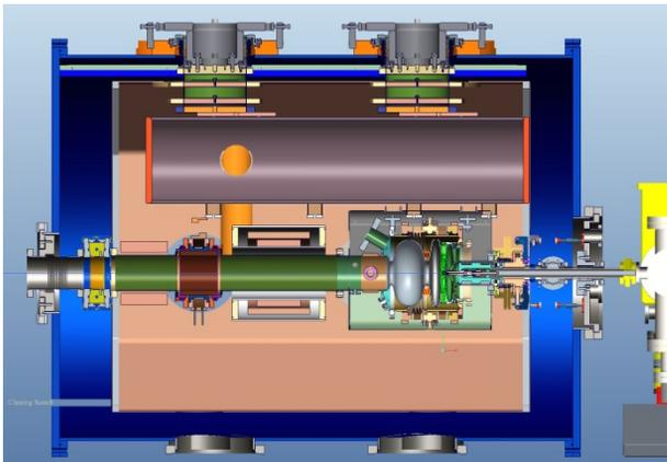
Figure 7: CAD view of the HZB SRF-gun structure assembled in a cryostat. (Courtesy HZB)
