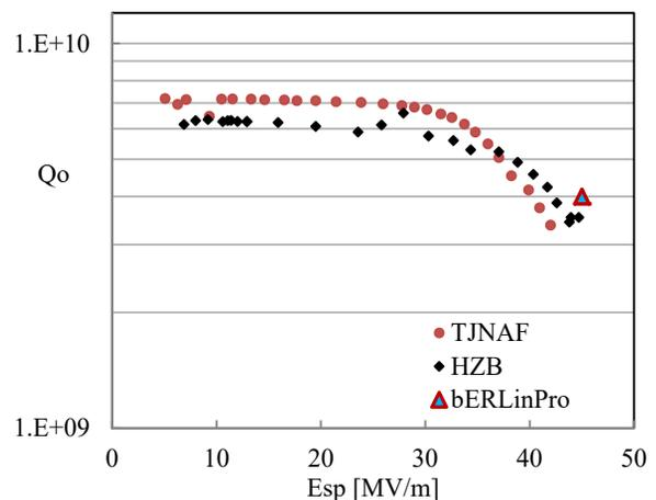
Figure 6:  $Q_0$  vs peak surface field  $E_{sp}$  as measured in vertical cryostat at TJNAF and at HZB at 1.8K.
