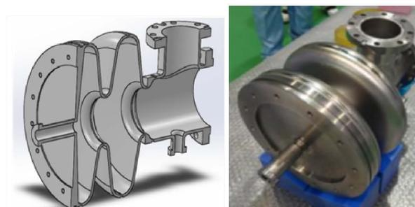
Figure 3: 1.3GHz prototype KEK cavity. (Courtesy KEK)
