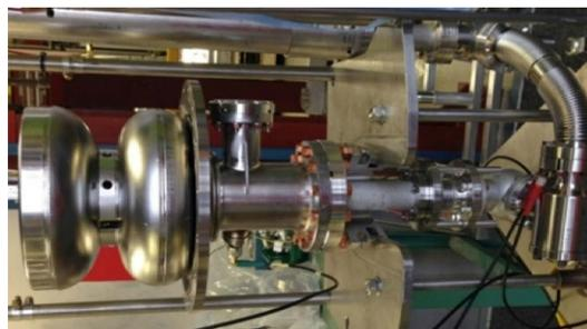
Figure 12: Prototype cavity in an insert, after electro-polishing and high-pressure water rinsing, prepared for the vertical test.
