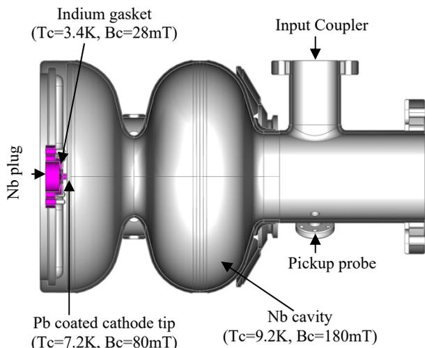
Figure 10: CAD drawing of the 1.6-cell DESY SRF-gun cavity with Nb-plug. Critical temperatures and magnetic flux for superconductors are shown in parenthesis.
