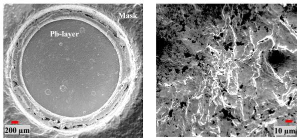
Figure 15: Pictures (not to scale) of the Pb-layer after the plasma treatment (left) and after the laser cleaning (right). *Courtesy NCBJ and BNL*
