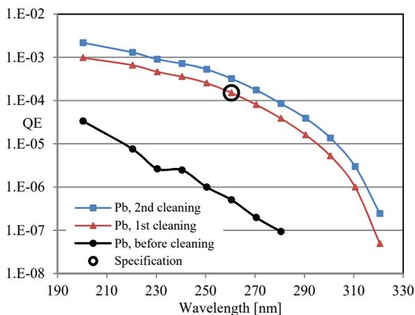
Figure 14: QE test results for of the Pb-layer deposited on the niobium plug at NCBJ. *Courtesy BNL*
