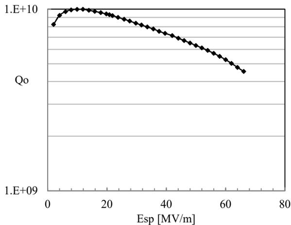
Figure 4:  $Q_0$  vs peak surface field  $E_{sp}$  measured at KEK in the first test at 1.7 K.
