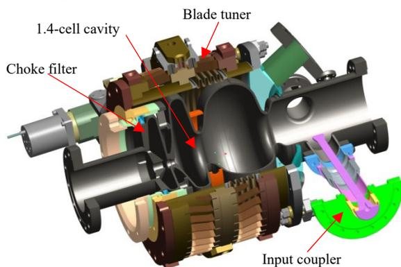
Figure 5: HZB SRF-gun structure equipped with a blade frequency tuner and an input coupler. (Courtesy HZB)
