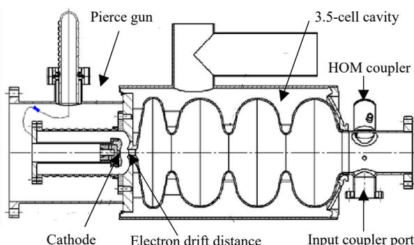
Figure 2: Drawing of DC Pierce gun and 3.5-cell PKU gun cavity. (Courtesy PKU)
