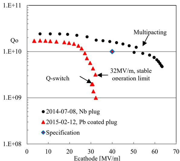
Figure 13: Recent test results for DESY SRF-gun cavity with the coated and uncoated plug. The shown multipacting could be processed in a short time.
