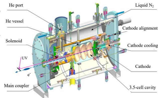
Figure 9: CAD drawing showing a cross section of the equipped Gun2 assembled in a cryostat. (Courtesy HZDR)
