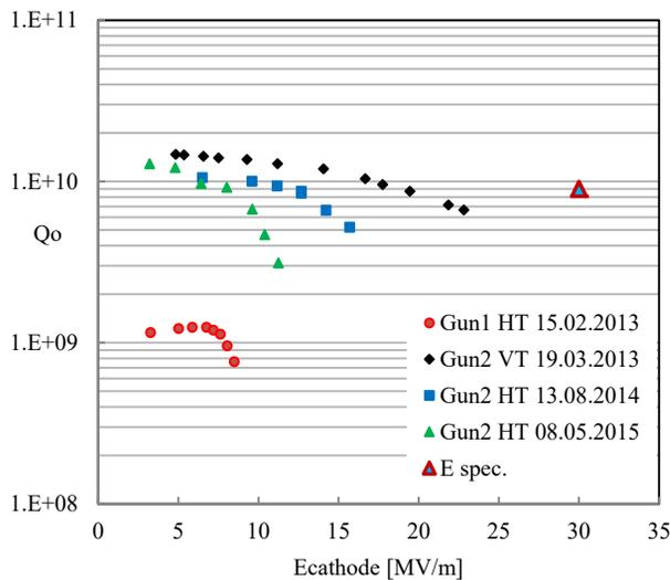
Figure 8: Tests results for Gun1 and Gun2 at TJNAF and at HZDR.
