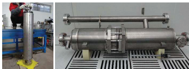
Figure 1: Cavity dressing with magnetic shield and helium vessel.
