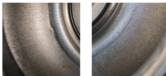
Figure 2: Macrostructures on cavity SPL #1.
