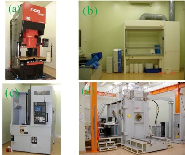
Figure 1: (a) Press machine, (b) CP area, (c) vertical lathe, (d) EBW machine, which are located in KEK-CFF.
