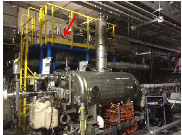
Figure 2: The 56 MHz cryomodule installed in the RHIC tunnel. Red arrow points to the quiet helium source tank.
