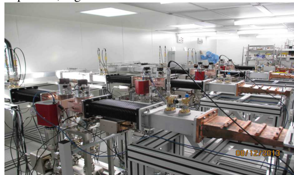
Figure 2: General layout of four channels for coupler conditioning.
