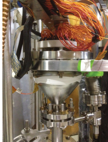
Figure 1: Third-generation Cornell TE sample host cavity with temperature map and external temperature sensors installed.
