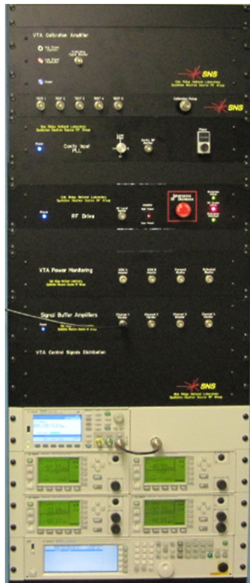
Figure 1: VTA RF Control System.
