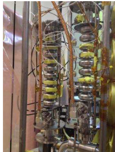
Figure 1: Vertical Insert with two cavities ready for Vertical Test, fully equipped with thermometers and Second Sound sensors.
