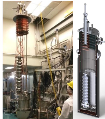
Figure 1: SRF test facility cavity cold test (left), cryostat section view (right).
