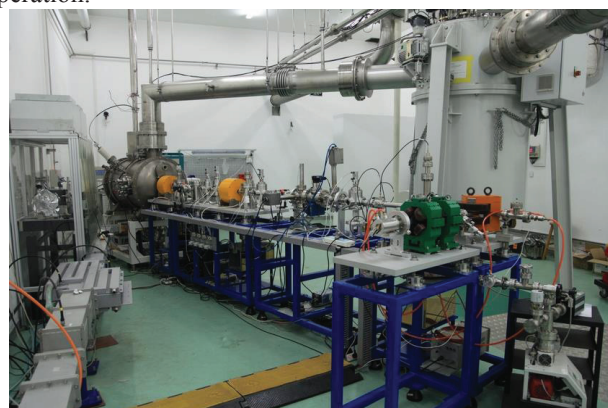
Figure 2: Beam experiment layout of the DC-SRF photoinjector.
