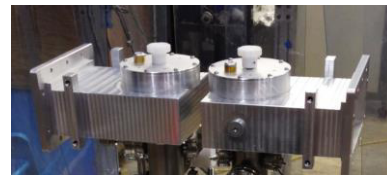
Figure 2: Pair of aluminium waveguide boxes being used for coupler RF processing.
