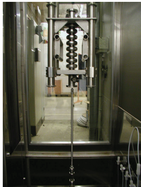
Figure 1: Undressed 3.9 GHz cavity in modified frame during high pressure rinsing.
