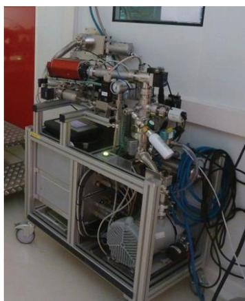
Figure 1: DESY Pumping group including SVPS unit at CEA, outside ISO4 cleanroom.
