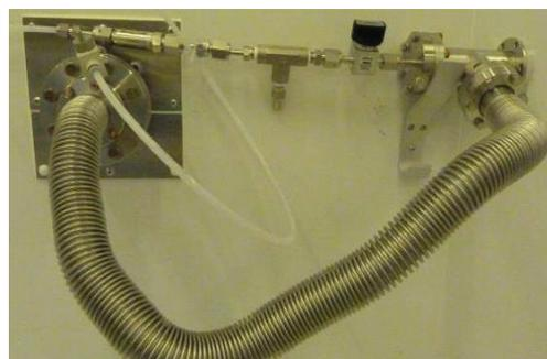
Figure 2: Connection of SVPS (behind the wall) and flushing unit inside cleanroom on the T part to be connected to the cavity (plastic cap on the flange).
