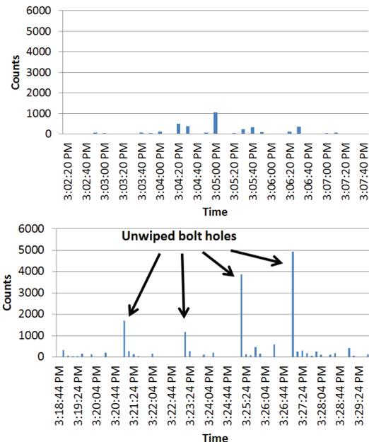
Figure 7: 0.3  $\mu\text{m}$  particle counts during cleaning of seal connections. A) Wiping bolt holes with cavity positioned horizontally; B) Bolt hole particle counts with and without wiping.
