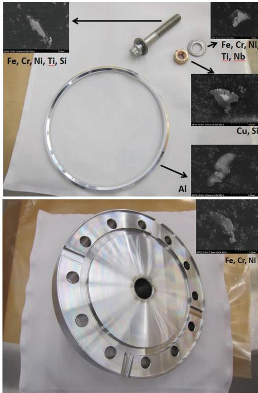
Figure 1: Particles found on assembly hardware after ultrasonic cleaning, before assembly.
