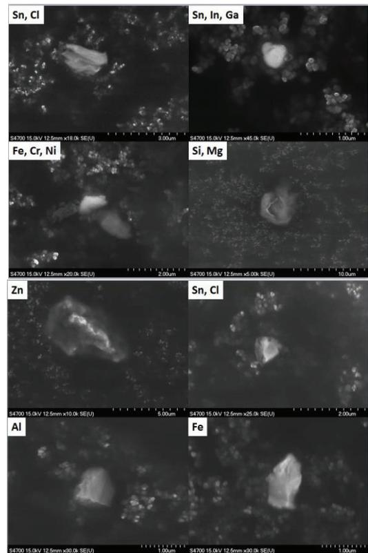
Figure 3: Particles found during horizontal assembly-disassembly experiment.
