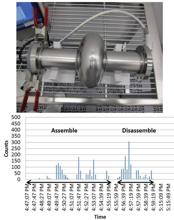
Figure 2: Horizontal assembly-disassembly setup and 0.3 μm particle counts.
