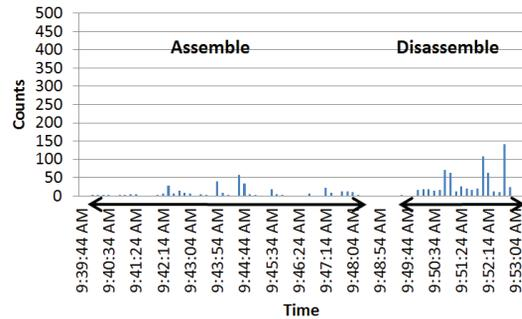
Figure 6: 0.3  $\mu\text{m}$  particle counts during vertical assembly-disassembly done by cleanroom assembly technician.
