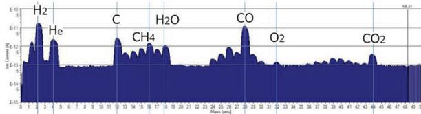
Figure 6: QMS analysis of desorption gases at ion pump baking.
