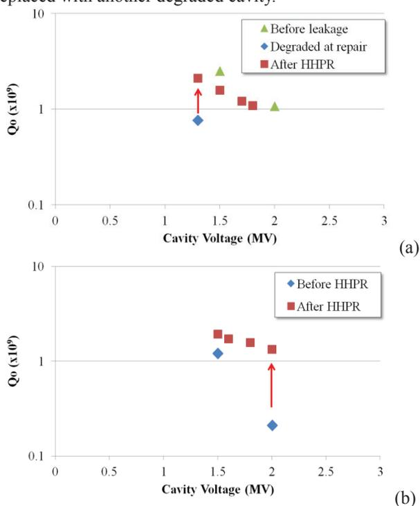
Figure 3:  $Q_0$  factors before and after HHPR. (a) The first HHPR cavity, (b) The second HHPR cavity.
