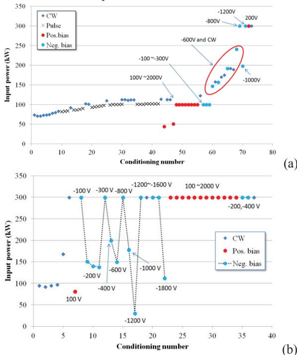
Figure 4: Coupler conditioning history. Input RF powers at the vacuum bursts are plotted in the order of conditioning number. No vacuum burst occurred when the RF power reached 300 kW. (a) The first HHPR cavity, (b) The second HHPR cavity.
