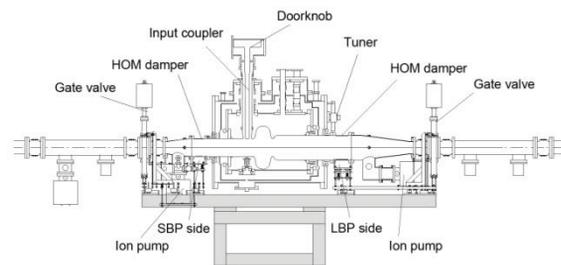
Figure 1: Cross-section of the SRF cavity module.
