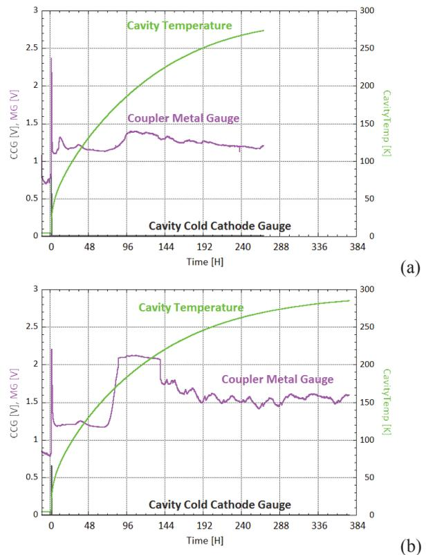
Figure 5: Vacuum pressure during warm-up. (a) The first HHPR cavity, (b) The second HHPR cavity.
