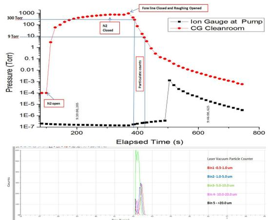
Figure 5: Purge and pump down particle data.
