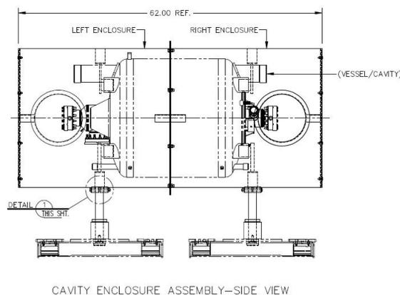
Figure 1: Schematic of the mock cryomodule side view.
