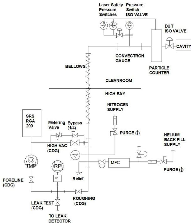
Figure 4: Clean room vacuum pump cart schematic.
