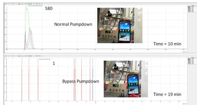
Figure 6: Comparison of pump down particle data, normal top and slow bottom.
