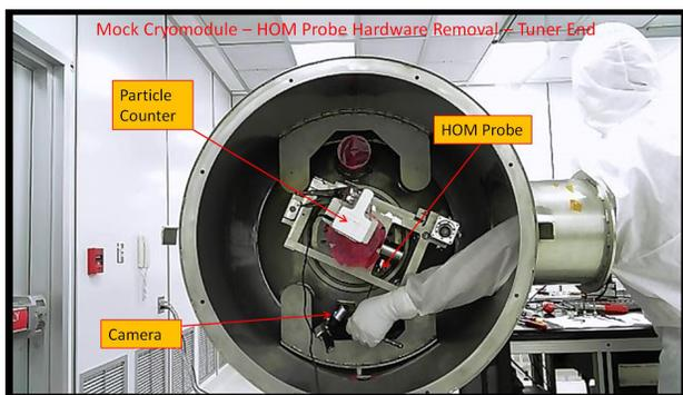
Figure 2: Mock cryomodule experimental setup.
