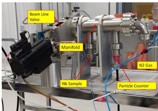
Figure 7: Beam line valve test setup.
