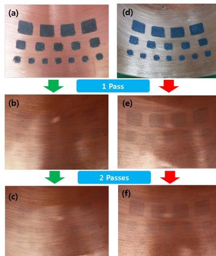
Figure 6: HPR Results with 100 bar of P@HPR: (a)-(c) show the surface states with the number HPR passes, the distance between a nozzle and a target is 30 mm, (d)-(f) show the surface states with the number HPR passes, the distance between a nozzle and a target is 170 mm.
