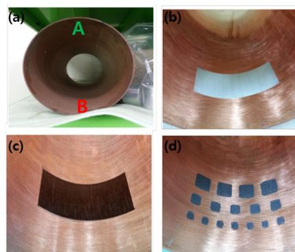
Figure 4: Various paintings on the simplified structure, painted area is  $100 \times 150 \text{ mm}^2$ : (a) A, B represents the part close to a nozzle as 30 mm and far from a nozzle as 170 mm, respectively, (b) inside view where painted by water-soluble board marker, (c) inside view where painted by permanent marker, and (d) inside view where painted with the pattern by water-soluble crayon.
