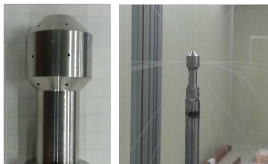
Figure 2: HPR Nozzle: nine holes on each top, middle, and bottom, angles of water sprays are 45 degrees.
