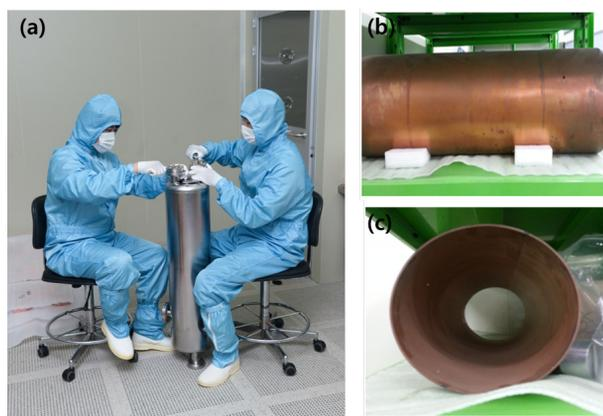
Figure 3: Simplified structure for HPR experiment, outer-conductor is separated from the cavity: (a) Nb half-wave resonator, (b) simplified structure (outer-conductor made of OFHC) of the actual cavity, and (c) the inside view with no painting.
