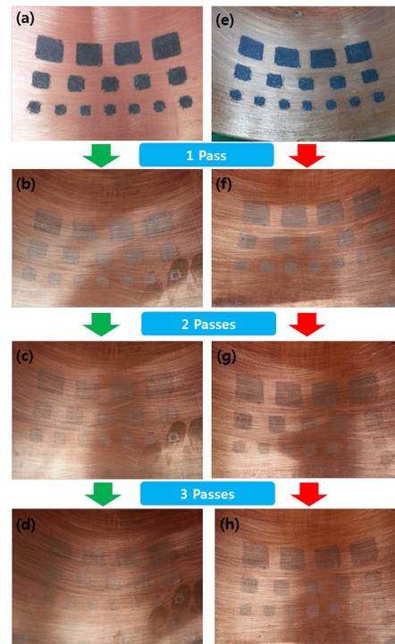
Figure 5: HPR Results with 60 bar of P@HPR: (a)-(d) show the surface states with the number HPR passes, the distance between a nozzle and a target is 30 mm, (e)-(h) show the surface states with the number HPR passes, the distance between a nozzle and a target is 170 mm.
