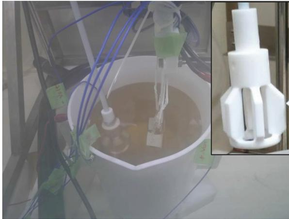
Figure 2: EP bath for lab EP experiments. Inset: Stirrer used in lab EP#2 and #3.
