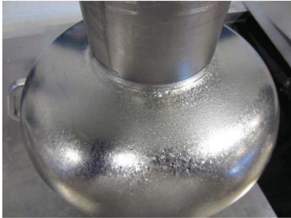
Figure 5: Significant grain growth observed in AES011.
