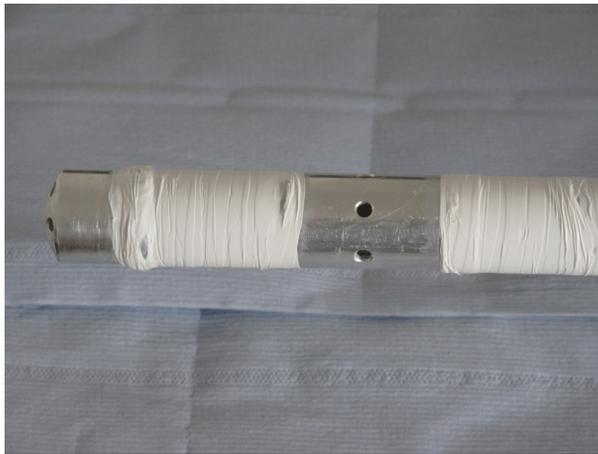
Figure 5b: View on acid injection holes and masking of electrode for 1.6 cell gun cavity vertical EP.
