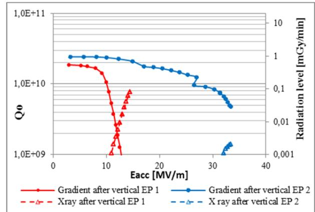
Figure 10: Test results of Gun cavity 16G2 after 1<sup>st</sup> and 2<sup>nd</sup> vertical EP.
