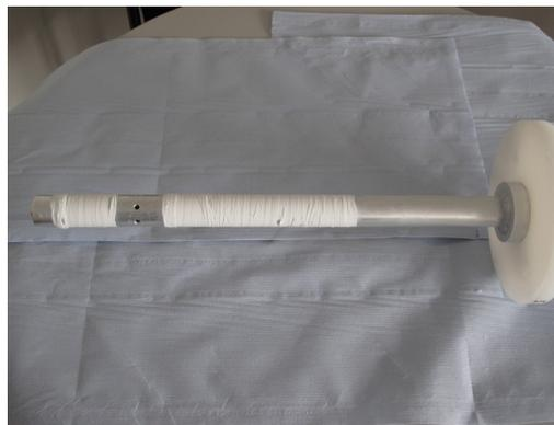
Figure 5a: Electrode for 1.6 cell gun cavity EP.
