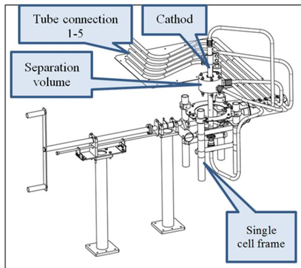
Figure 1: Design drawing of frame work for vertical EP.
