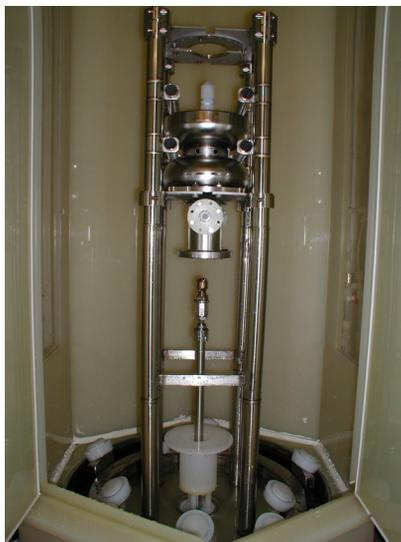
Figure 9: Gun cavity 16G2 installed to HPR stand.
