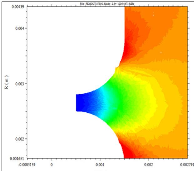
Figure 6: Contour of the electrical field amplitude at plug.
