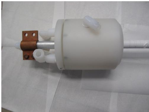
Figure 2: Separation volume for vertical EP with electrode installed.
